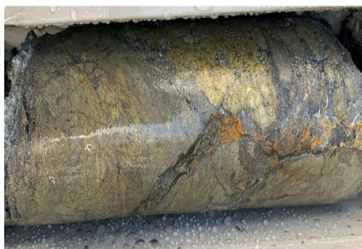
Figure 5: sample from CRR21DD_04 exhibiting extensive massive sulphide with abundant brassy yellow chalcopyrites
