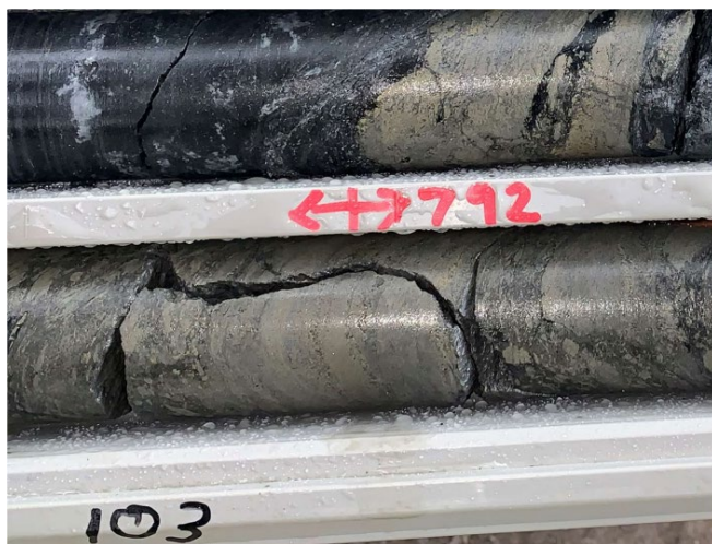
Figure 4: sample from CRR21DD_04 exhibiting extensive massive sulphide (some brecciated)
