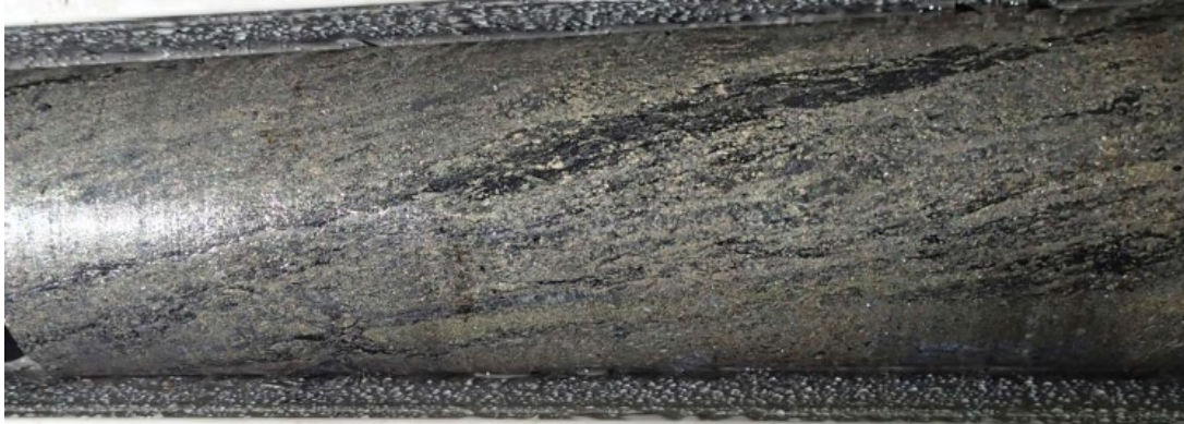
Figure 5: sample from CRR21DD_14 exhibiting extensive banded, massive sulphide
