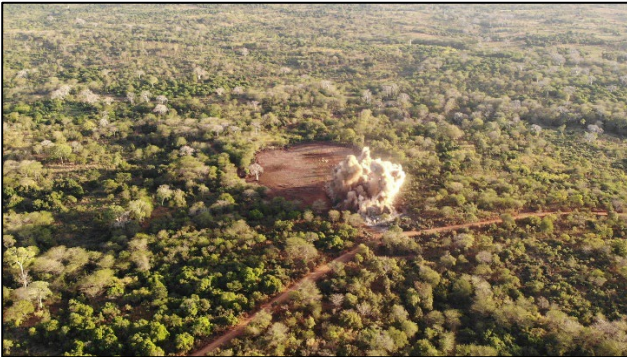
Figure 5: First blast at the starter pit (left) and loading and hauling (right). Note the high-grade graphite stockpile in the background.
