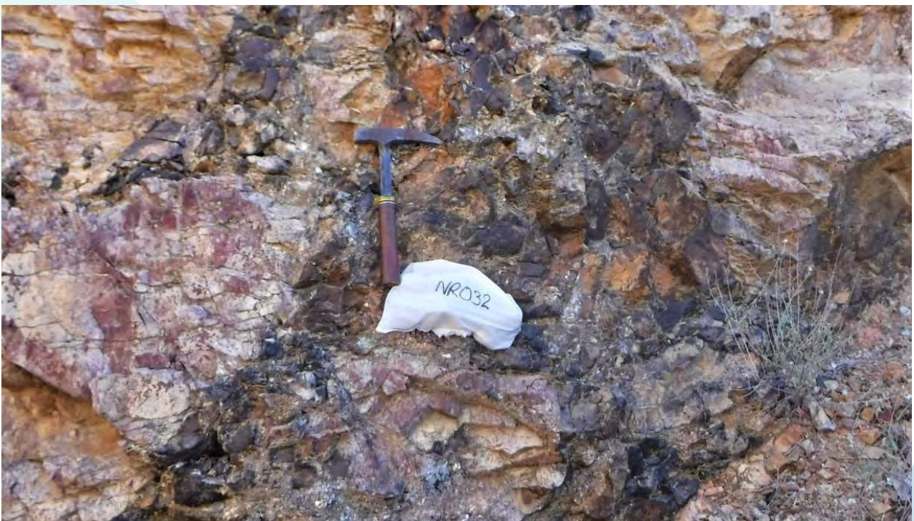
Figure 4: Pit wall of quarry at site 19a with abundant lithium phosphate minerals (dark brown to purple-black mineral) sampled as NR032.
