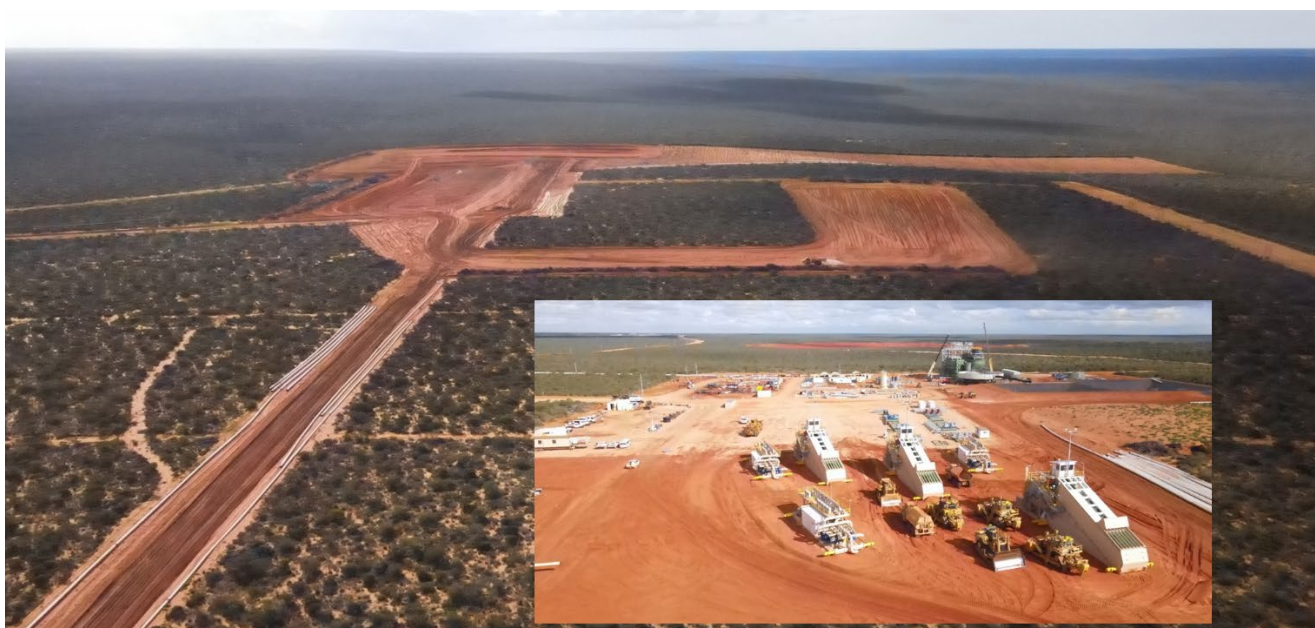
Figure 6 Development of open mine pits & three dozer mining units (DMU's) ready to be moved into position for mining first ore
