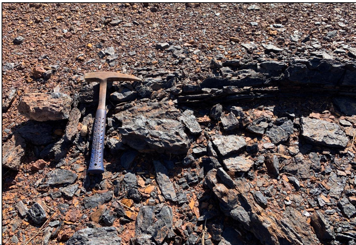
Figure 2 - Manganese replacement of laminated shale at Manganese Area 3 - WR0018Mn - 36.1 % Mn from laboratory analysis (previously 26.2% Mn from pXRF)
