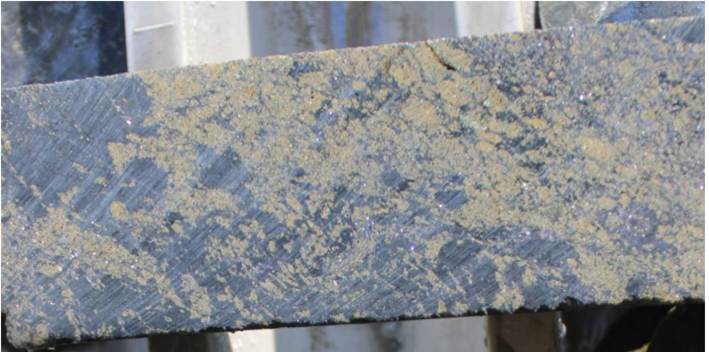
Figure 7c: CRR21DD_018, Portion of sample 43010 above, core sawn longitudinally to exhibit abundant sphalerite (zinc sulphide, pale cream-light yellow brown ) and galena (lead sulphide, silvery-grey) in black carbonaceous pelite (NQ core, 50mm diameter)
