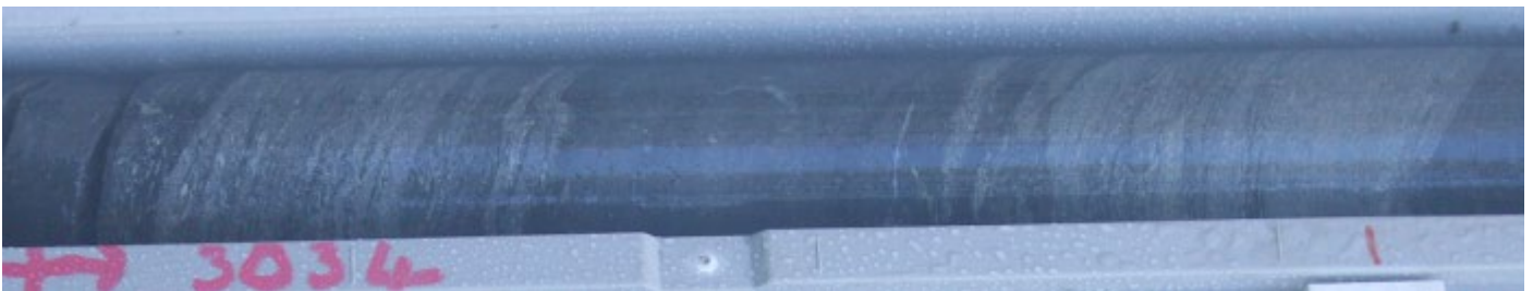
Figure 11: CRR21DD_018, Portion of sample 43034 (191.15-191.80m downhole) sub-parallel base metal beds with sphalerite (zinc sulphide, pale cream-light yellow brown) and lesser galena (lead sulphide, silvery-grey) in black carbonaceous pelite - sample assayed 7.70% Zn, 4.58% Pb, 1.15% Cu, 112g/t Ag and 0.38g/t Au, part of the longer downhole interval of 8.00m @ 4.59% Zn, 1.65% Pb, 0.70% Cu, 98.63g/t Ag and 0.21g/t Au from 183.80-191.80m downhole (NQ core, 50mm diameter)
