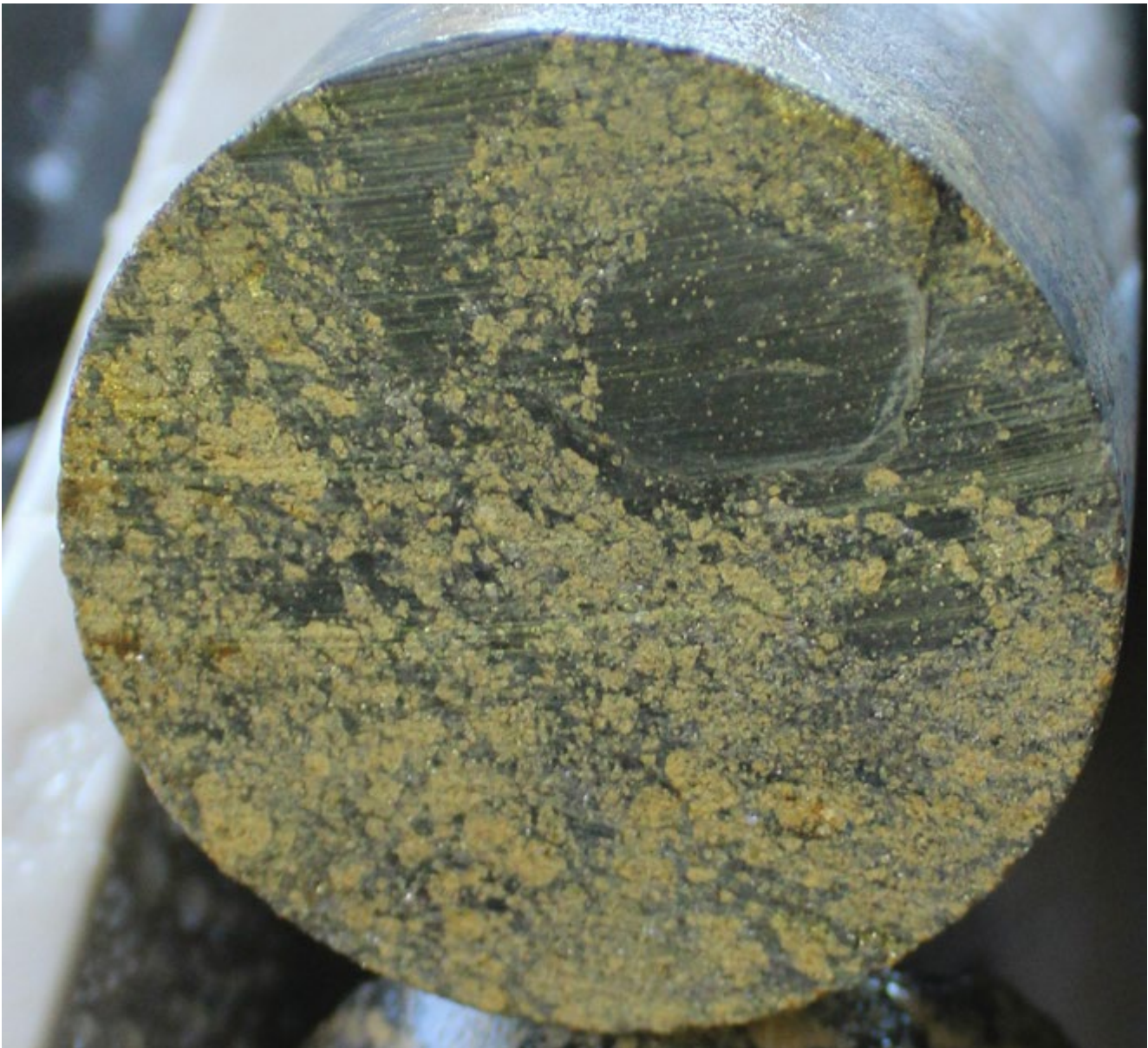
Figure 7b: CRR21DD_018, Portion of sample 43010 above, core sawn transversely to exhibit abundant sphalerite (zinc sulphide, pale cream-light yellow brown ) in black carbonaceous pelite (NQ core, 50mm diameter)
