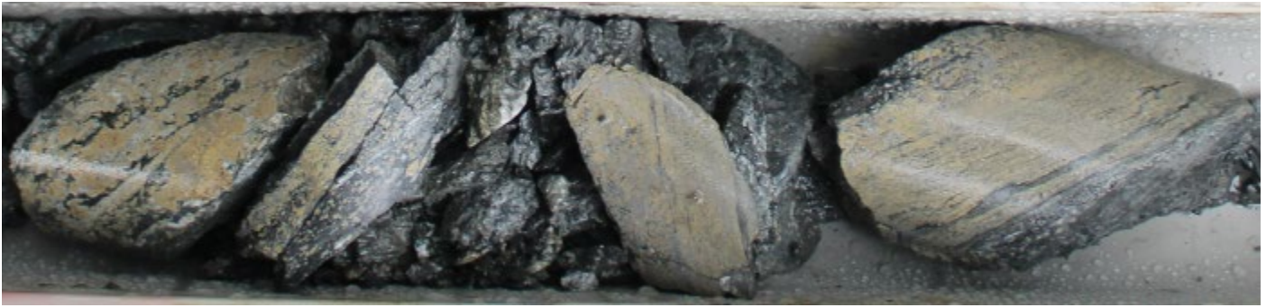
Figure 2: CRR21DD_018, Portion of sample 42951 (65.51-66.51m downhole) exhibiting beds of massive sulphides – sphalerite (zinc sulphide, pale cream-light yellow brown) and lesser galena (lead sulphide, silvery-grey) in black carbonaceous pelite - sample assayed 9.41% Zn, 3.47% Pb, 0.25% Cu, 15.75g/t Ag and 0.10g/t Au (NQ core, 50mm diameter)
