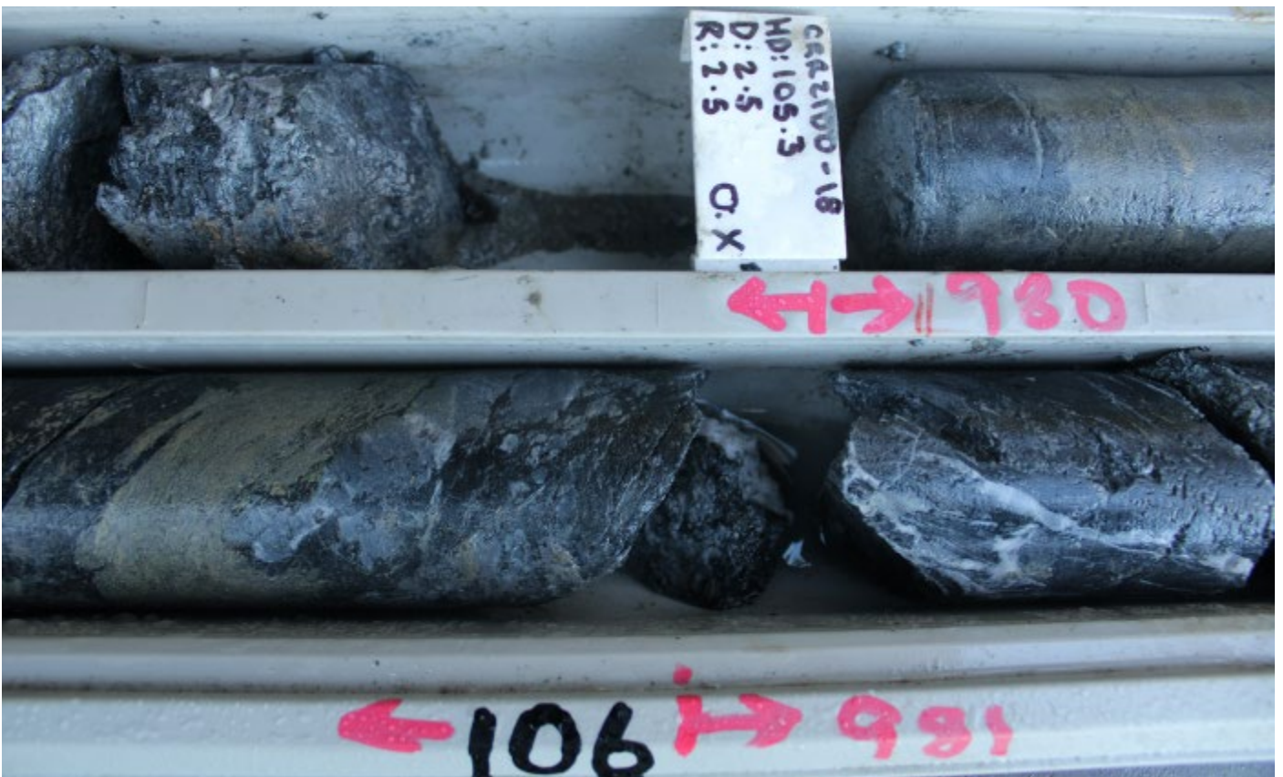
Figure 5: CRR21DD_018, Portion of sample 42980 (105.30-106.00m downhole) exhibiting beds of massive sulphides – sphalerite (zinc sulphide, pale cream-light yellow brown ) and chalcopyrite (copper-iron-sulphide, brassy-yellow), galena (lead sulphide, silvery-grey) in black carbonaceous pelite - sample assayed 21.50% Zn, 9.60% Pb, 3.45% Cu, 44g/t Ag and 0.33g/t Au, part of the longer downhole interval of 18.41m @ 2.37% Zn, 0.91% Pb, 0.48% Cu, 24.34g/t Ag and 0.07g/t Au from 88.09-106.50m downhole (including 3.7m @ 6.06% Zn, 2.41% Pb, 1.39% Cu, 22.08g/t Ag, 0.16g/t Au from 102.8-106.5m downhole (NQ core, 50mm diameter)
