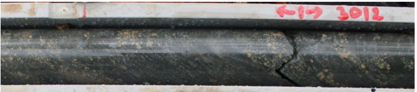
Figure 8: CRR21DD_018, Portion of sample 43012 (153.57-155.37m downhole) exhibiting sub-parallel discontinuous beds with blebs sphalerite (zinc sulphide, pale cream-light yellow brown) and lesser galena (lead sulphide, silvery-grey ) in black carbonaceous pelite - sample assayed 7.28% Zn, 1.67% Pb, 0.18% Cu, 16.90g/t Ag and 0.13g/t Au, part of the longer downhole interval of 7.47m @ 4.61% Zn, 1.57% Pb, 0.17% Cu, 39.73g/t Ag and 0.09g/t Au from 147.90-155.37m downhole (NQ core, 50mm diameter)
