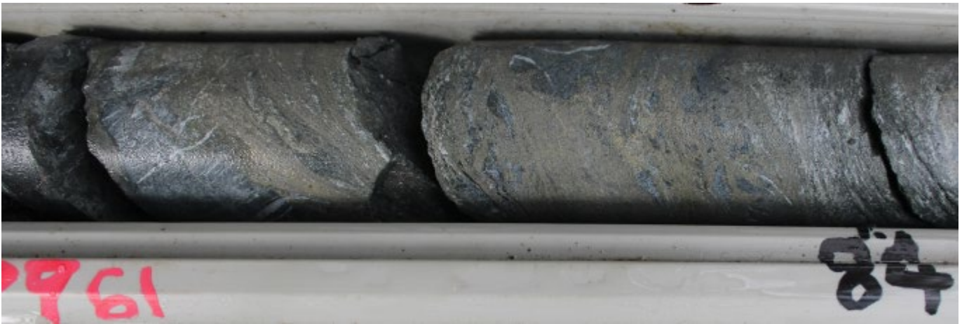
Figure 3: CRR21DD_018, Portion of sample 42961 (83.77-84.09m downhole) exhibiting beds of massive sulphides – sphalerite (zinc sulphide, pale cream-light yellow brown) and lesser galena (lead sulphide, silvery-grey) in black carbonaceous pelite - sample assayed 17.65% Zn, 9.53% Pb, 1.36% Cu, 172g/t Ag and 0.67g/t Au (NQ core, 50mm diameter)
