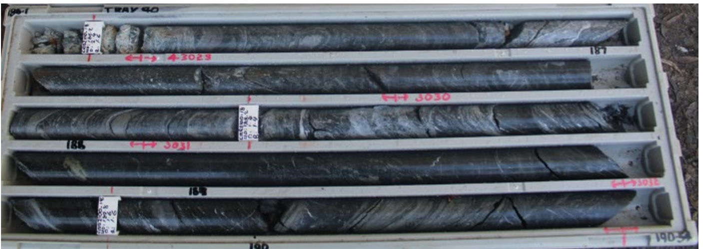
Figure 9: CRR21DD_018, diamond core from 186.10m-190.54m part of an interval part of the longer downhole interval of 8.00m @ 4.59% Zn, 1.65% Pb, 0.70% Cu, 98.63g/t Ag and 0.21g/t Au from 183.80-191.80m downhole (NQ core, 50mm diameter)
