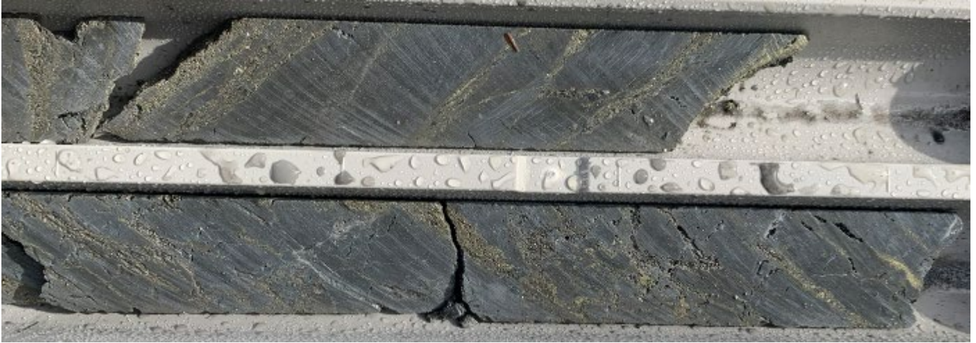
Figure 13: CRR21DD_011B, Portion of sample 43075 (43.20-44.80m downhole) exhibiting sheeted veins of pyrite and lesser chalcopyrites (copper sulphide mineral) – sample assayed 1.54% Cu, 0.36% Zn and 105g/t Ag (NQ core, 50mm diameter)
