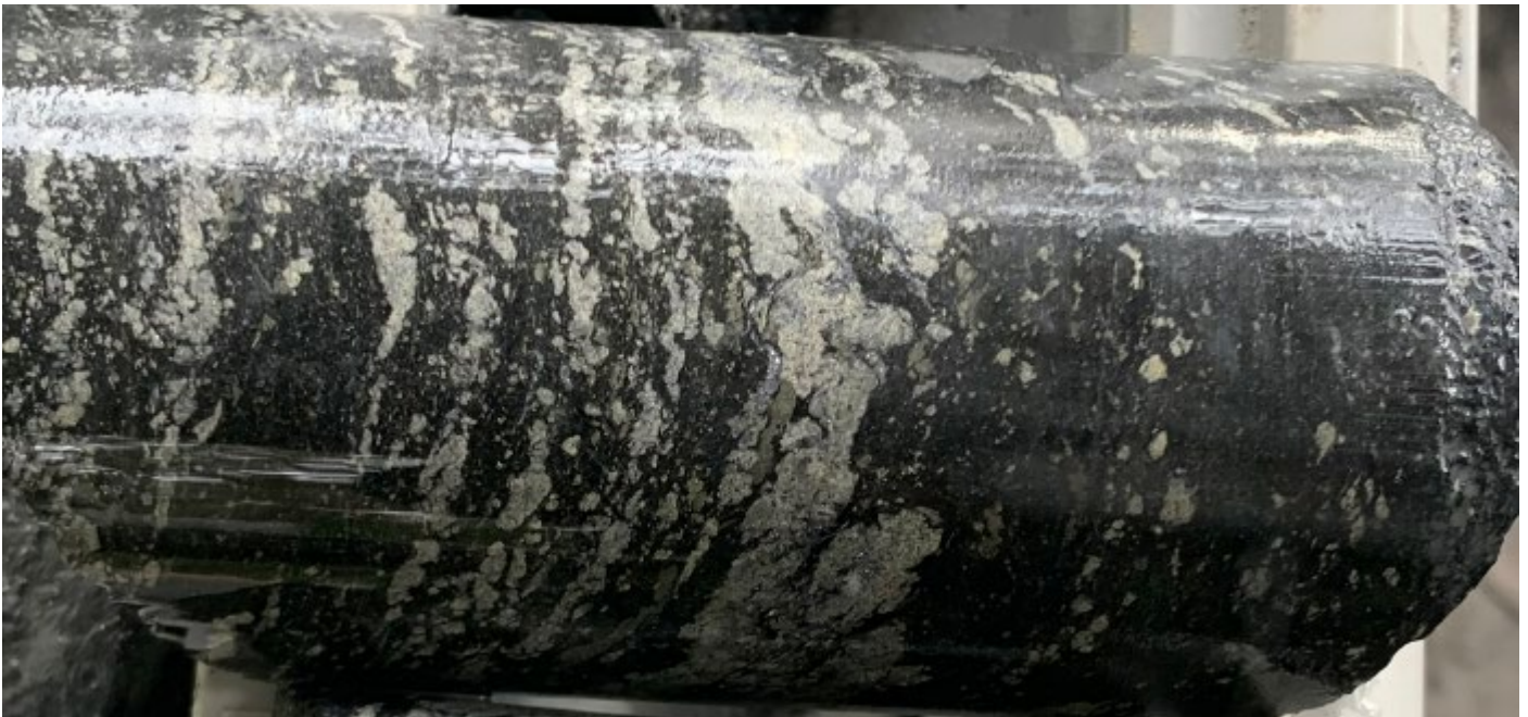
Figure 12: CRR21DD_017, Portion of sample 42880 (26.30-27.30m downhole) exhibiting sub-parallel discontinuous beds of base metal sulphides – sphalerite (zinc sulphide, pale cream-light yellow brown ) and lesser galena (lead sulphide, silvery-grey) in black carbonaceous pelite - sample assayed 11.35% Zn, 5.96% Pb, 0.50% Cu, 50.8g/t Ag and 0.03g/t Au, part of the longer downhole interval of 7.20m @ 3.74% Zn, 1.77% Pb, 0.15% Cu, 18.17g/t Ag from 25.10-32.30m downhole (NQ core, 50mm diameter)
