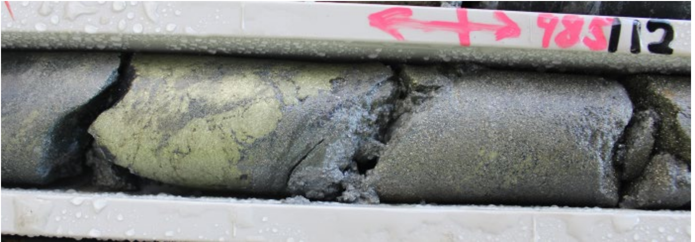
Figure 6a: CRR21DD_018, Portion of sample 42985 (111.95-113.50m downhole) exhibiting abundant brassy-yellow chalcopyrite (copper-iron-sulphide) - sample assayed 2.95% Cu (NQ core, 50mm diameter)
