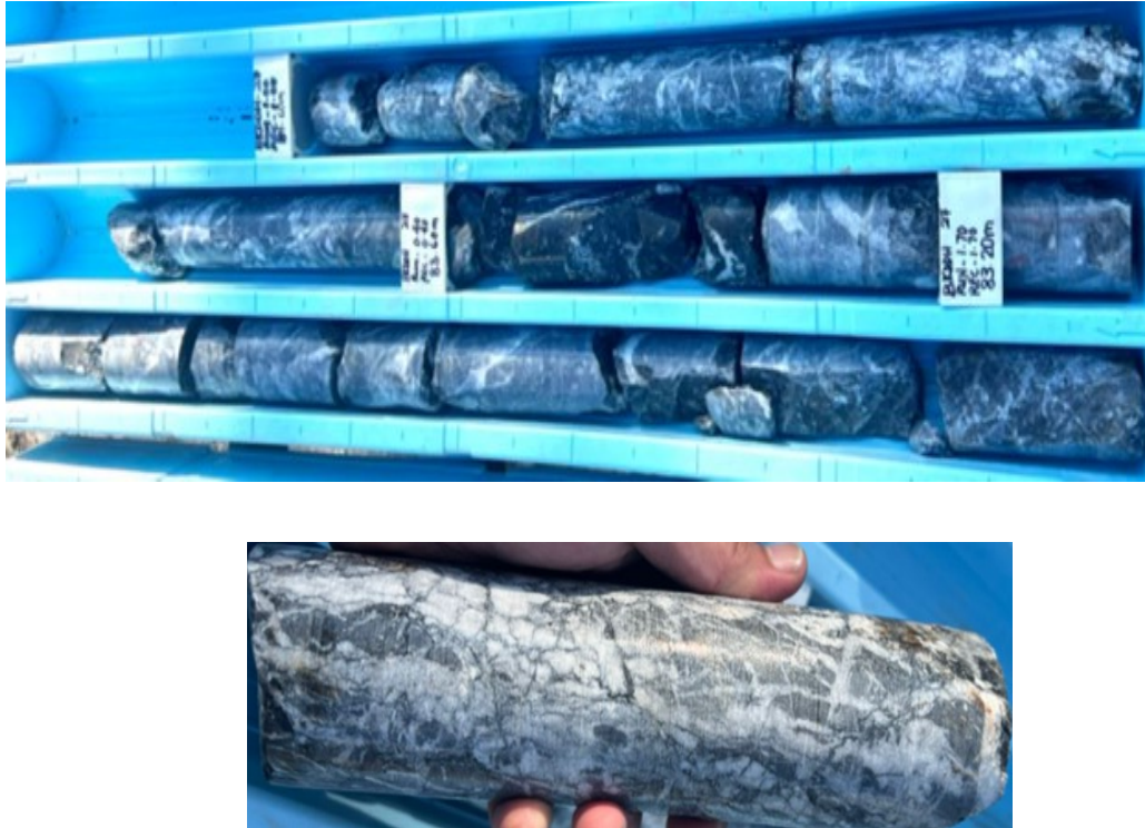
Figure 13: Section BKDDH-26, illustrating the intensely hydrothermally altered Bau Limestone, typical of textures endowed with higher grade gold mineralisation along trend at the former Tai Parit and BGY mines.
