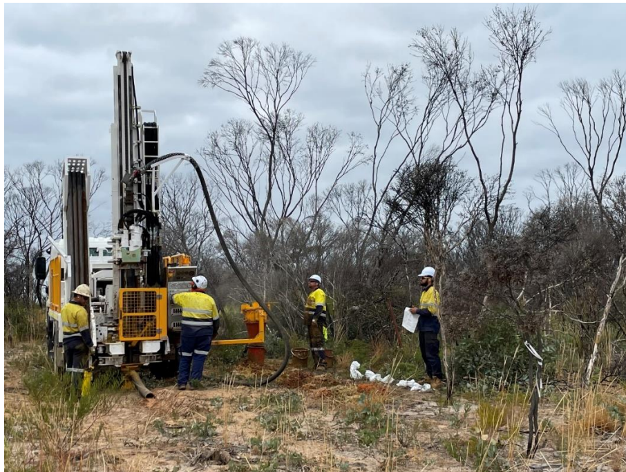
Photograph 1: Aircore drilling at the Mount Ridley Project.
