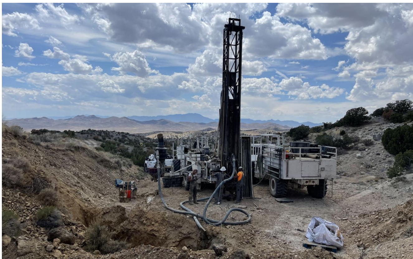
Figure 1: Reverse circulation drilling rig setting up to commence drilling hole 3MZRC22-001 at Mizpah.
