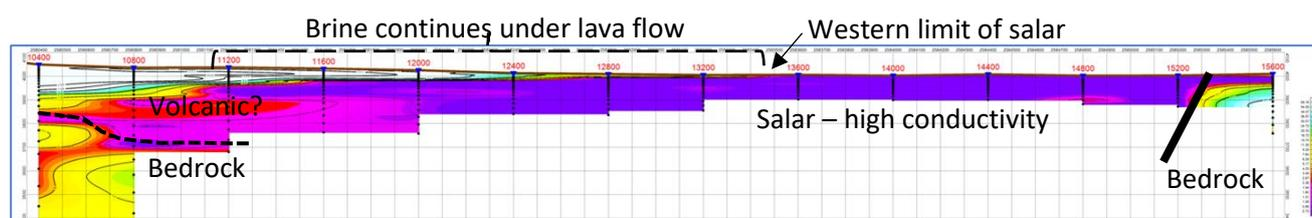
Figure 4: Cross section along TEM line 6, showing the extension of brine (pink to blue zones) beneath lava flows west of the salar
