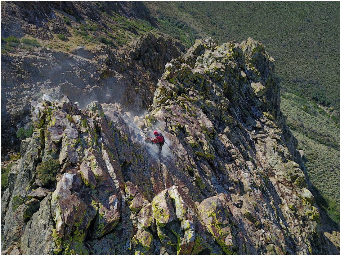
Figure 5. PolarX field crew saw-cutting channel sample across vein swarms at the Golden Staircase target, Humboldt Range, Nevada.
