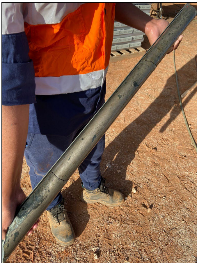
Figure 1: Part of the 3.6m lens of massive nickel sulphide intersected in TED41. See text for further details.
