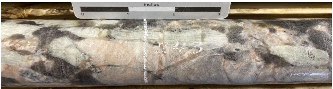
Figure 1: Close up of MF22-118 at 243-243.1m downhole. Significant white-grey large spodumene laths
