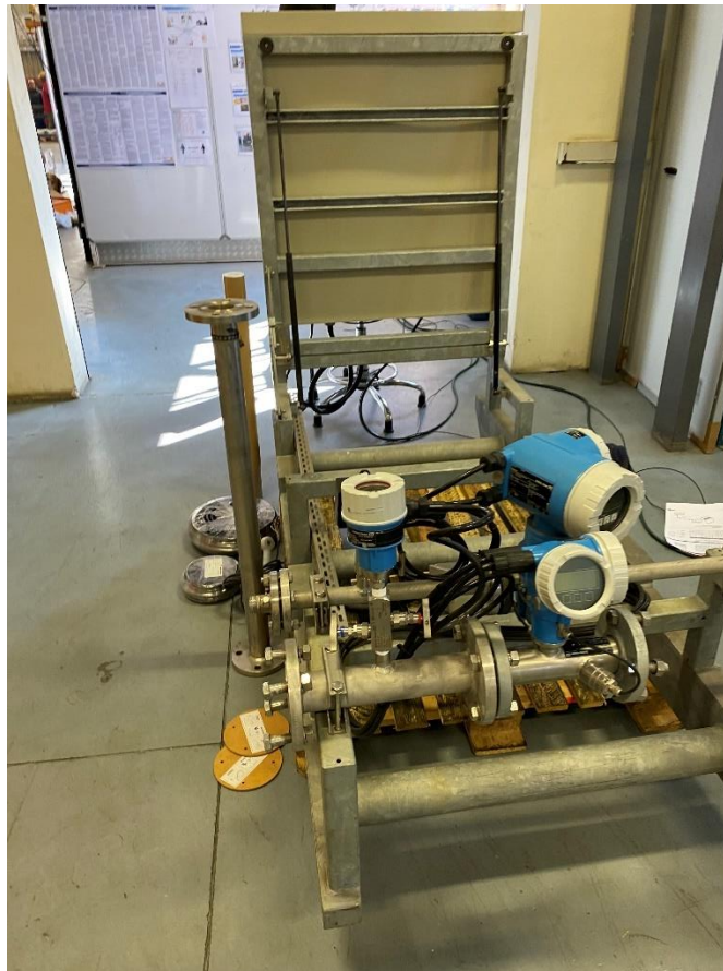
Figure 2 - Serowe 3 Flow Testing Skid post factory testing at Franklin Electric (Pty) Ltd facility in South Africa.
