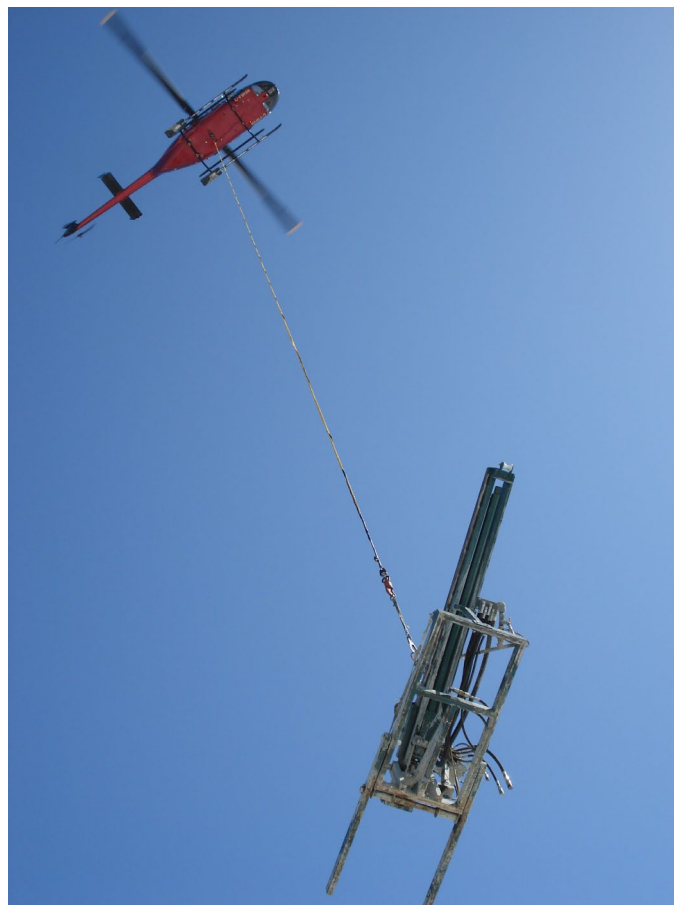
Figure 6 – RC Drill rig being transported by helicopter
