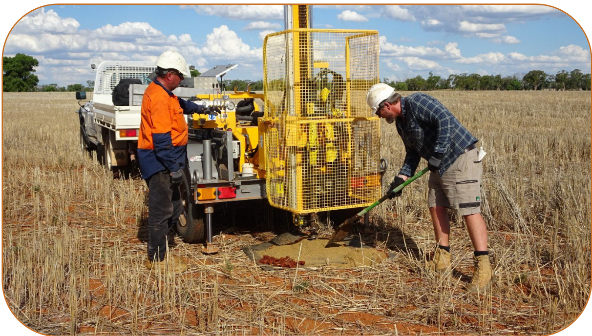
Figure 2: Typical small, scale Auger Rig in action (Source IMEx – with thanks)
