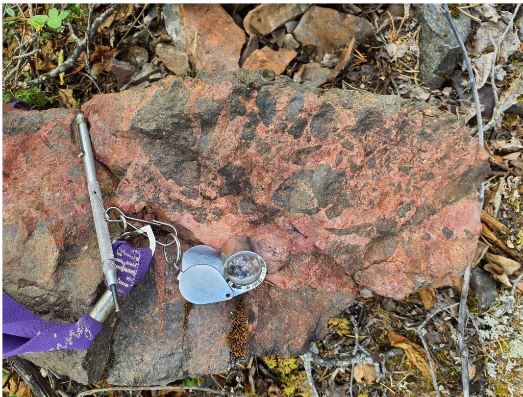
Figure 1: Surprise Creek Fault - Hematitic breccia with U, Cu and Pb mineralisation (max scintillometer reading of 65,535 cps)
