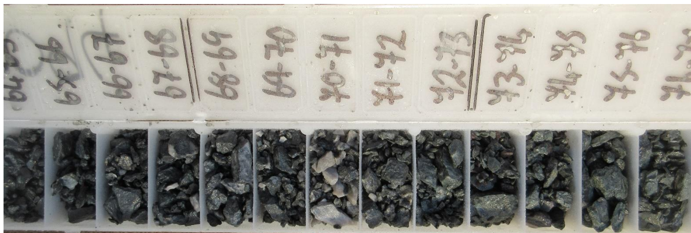
Figure 3 GCRC094 (68 – 73m downhole intercept mineralised zone)
