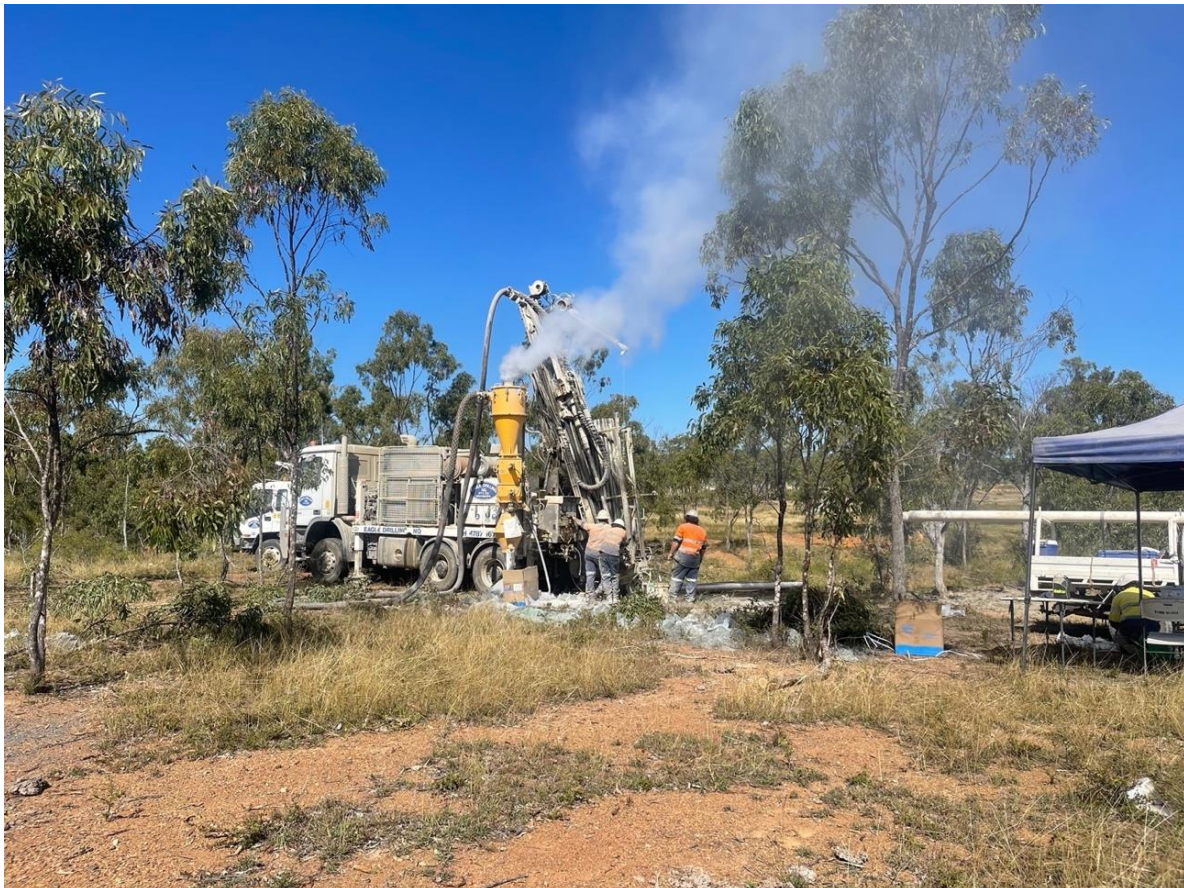
Figure 1 RC drill rig drilling at Golden Cup
