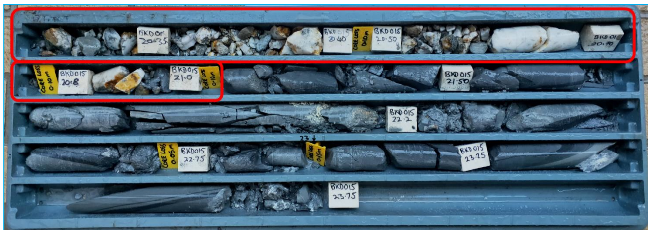
Figure 2: Diamond drillhole BKD015 - High-Grade, Quartz-Hosted Gold Intercept Outlined (20.2 – 21.0m, 0.80m @ 19.2 g/t Au including 0.30m @ 27.0 g/t Au from 20.2m)
