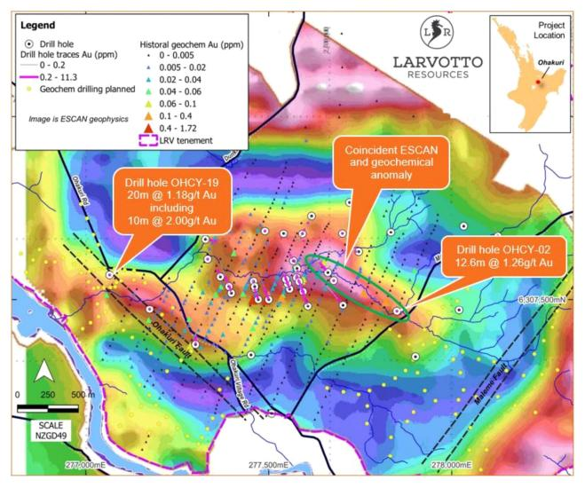
Figure 1 ESCAN geophysics with drilling
