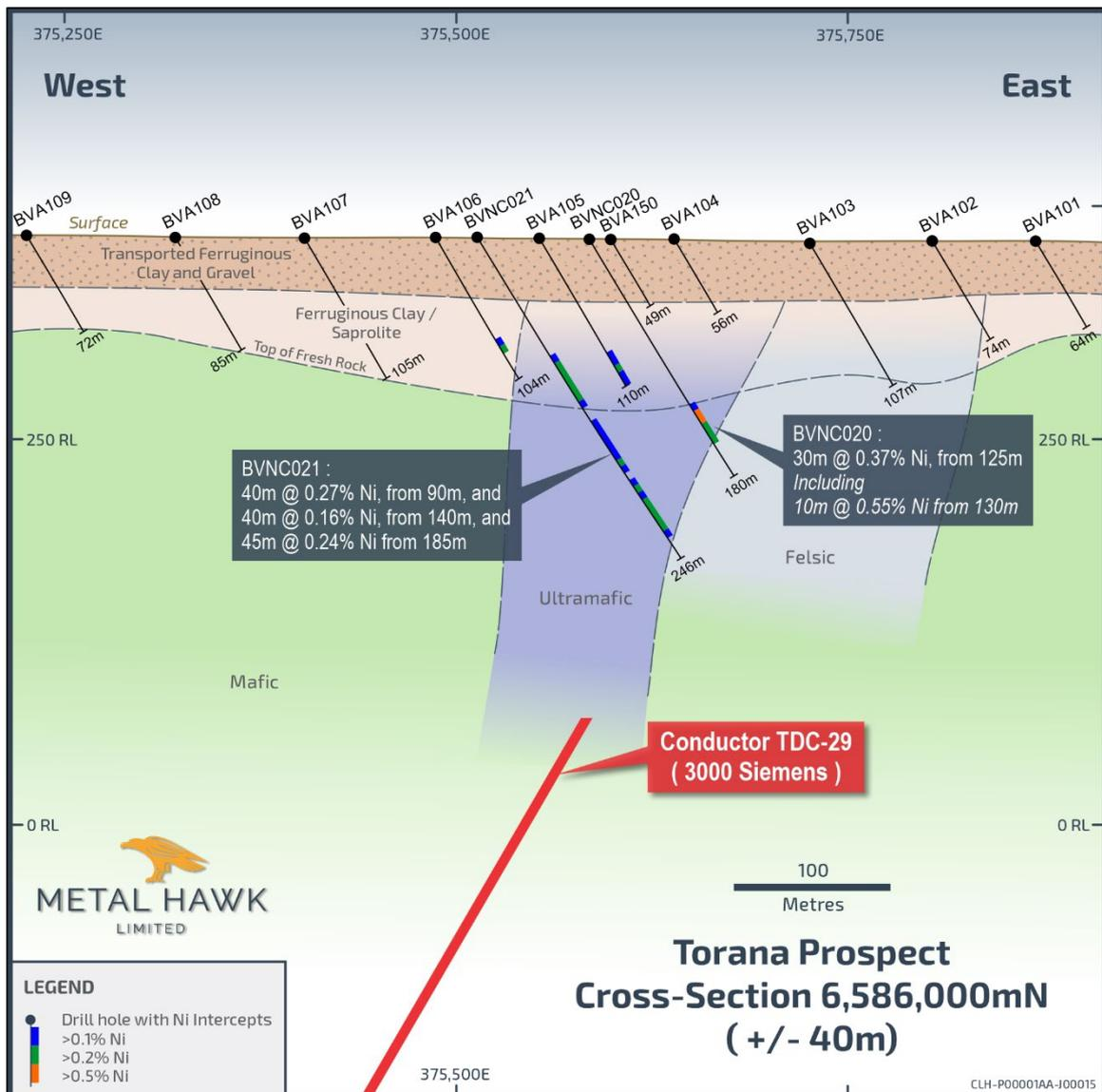
**Figure 1.** Cross section 6,586,000mN showing DHEM conductor plate TDC\_29.
