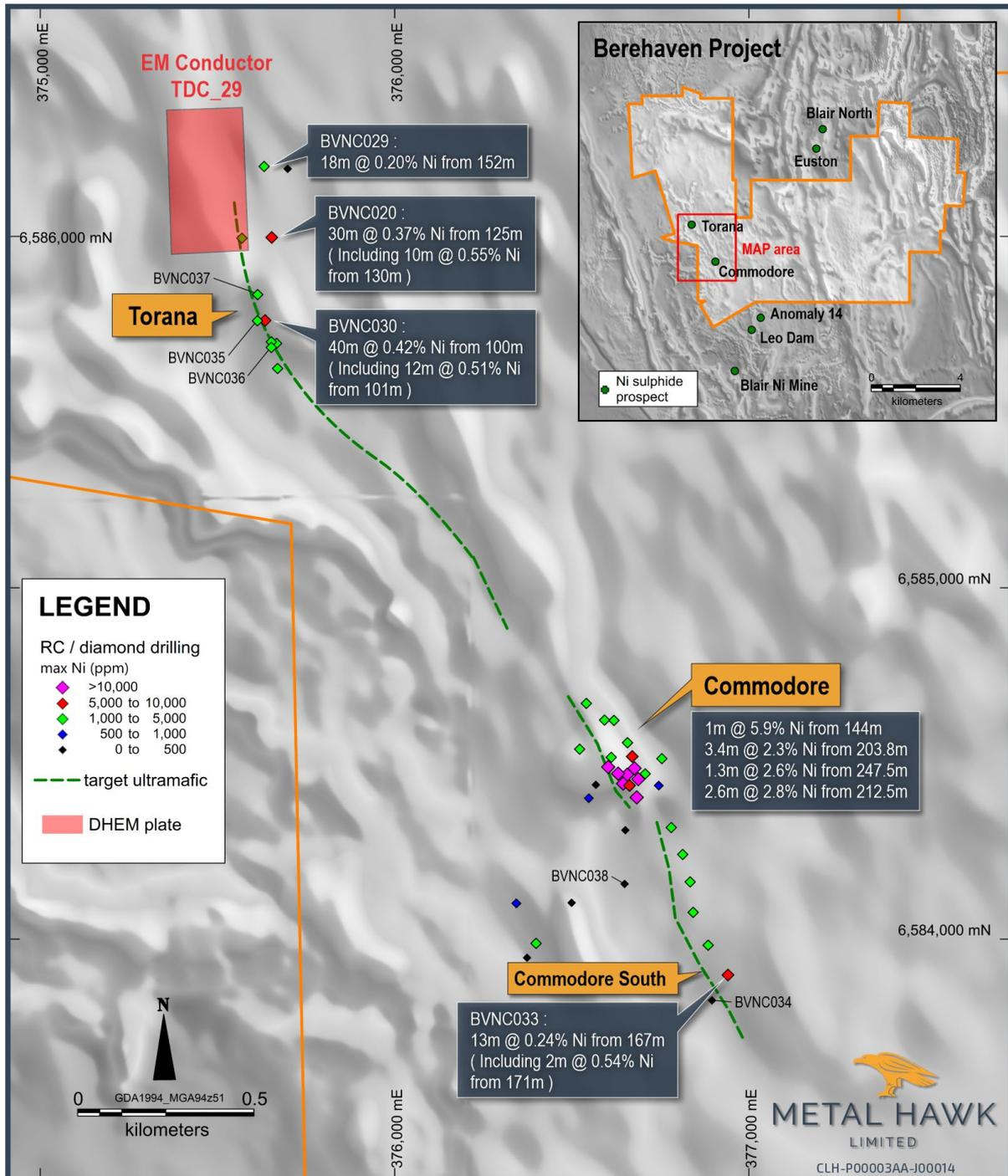
**Figure 2.** Commodore drill plan over airborne magnetics showing RC and diamond drilling with highlights, new hole locations and DHEM conductor plate **TDC\_29**
