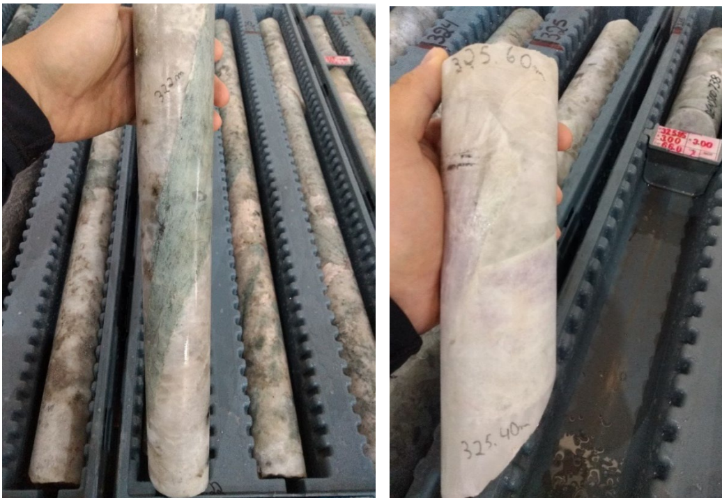
Figure 1: SADD033 – Spodumene rich pegmatite over 18.75m down hole thickness (321.15-339.90m)
