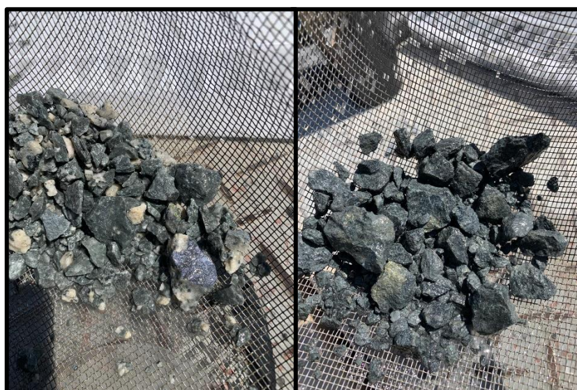
Figure 3. Bommie Prospect: Drill chips showing albite, chlorite, biotite, disseminated sulphides and quartz-carbonate veins.
