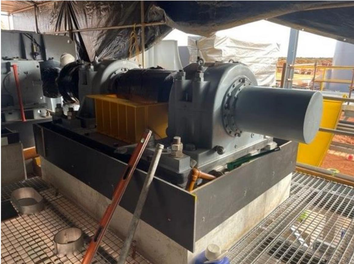
**Figure 7** – Mill pinion drive.
