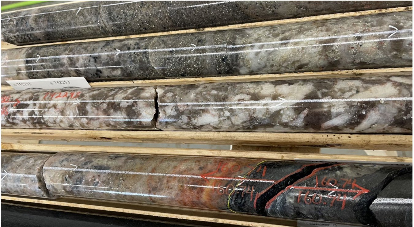
Figure 1: MF22-73 spodumene-bearing pegmatite zone (149.90 to 160.74m downhole) with lower contact with the mafic volcanic unit
