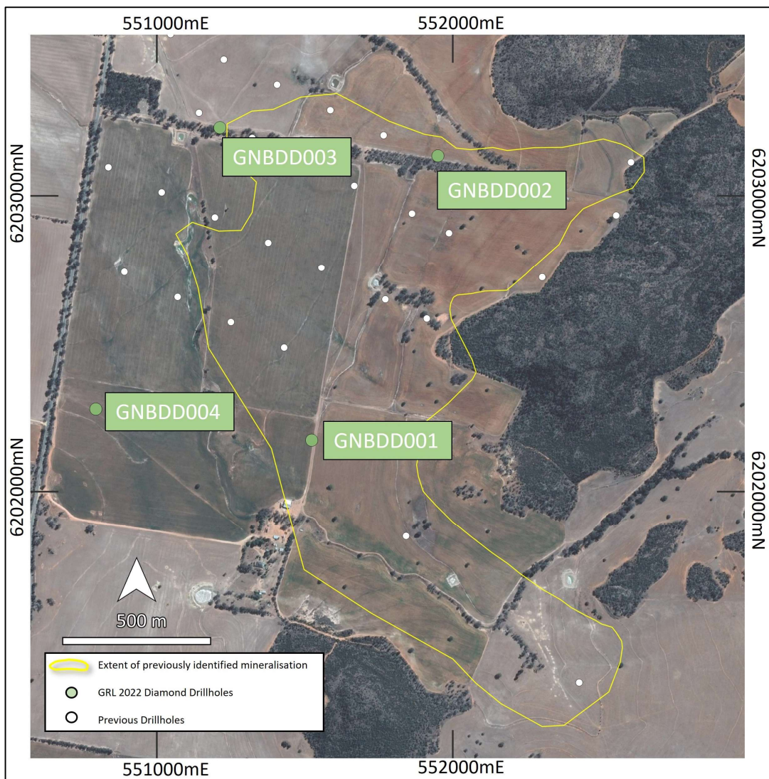
Figure 1: Location of the four diamond drill holes at Narraburra.
