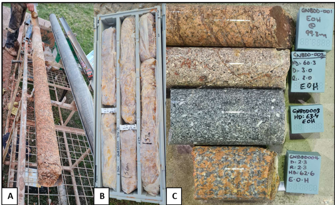
Figure 3: A: Photo of weathered drill core in splits B: Clay wrapped in plastic to retain moisture. C: End of hole fresh rock samples.
