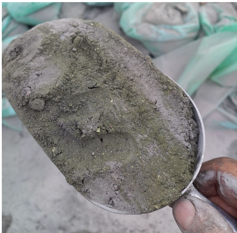
Photo 1. Un-sieved example of MHRC025 copper sulphides from 285-286m.
