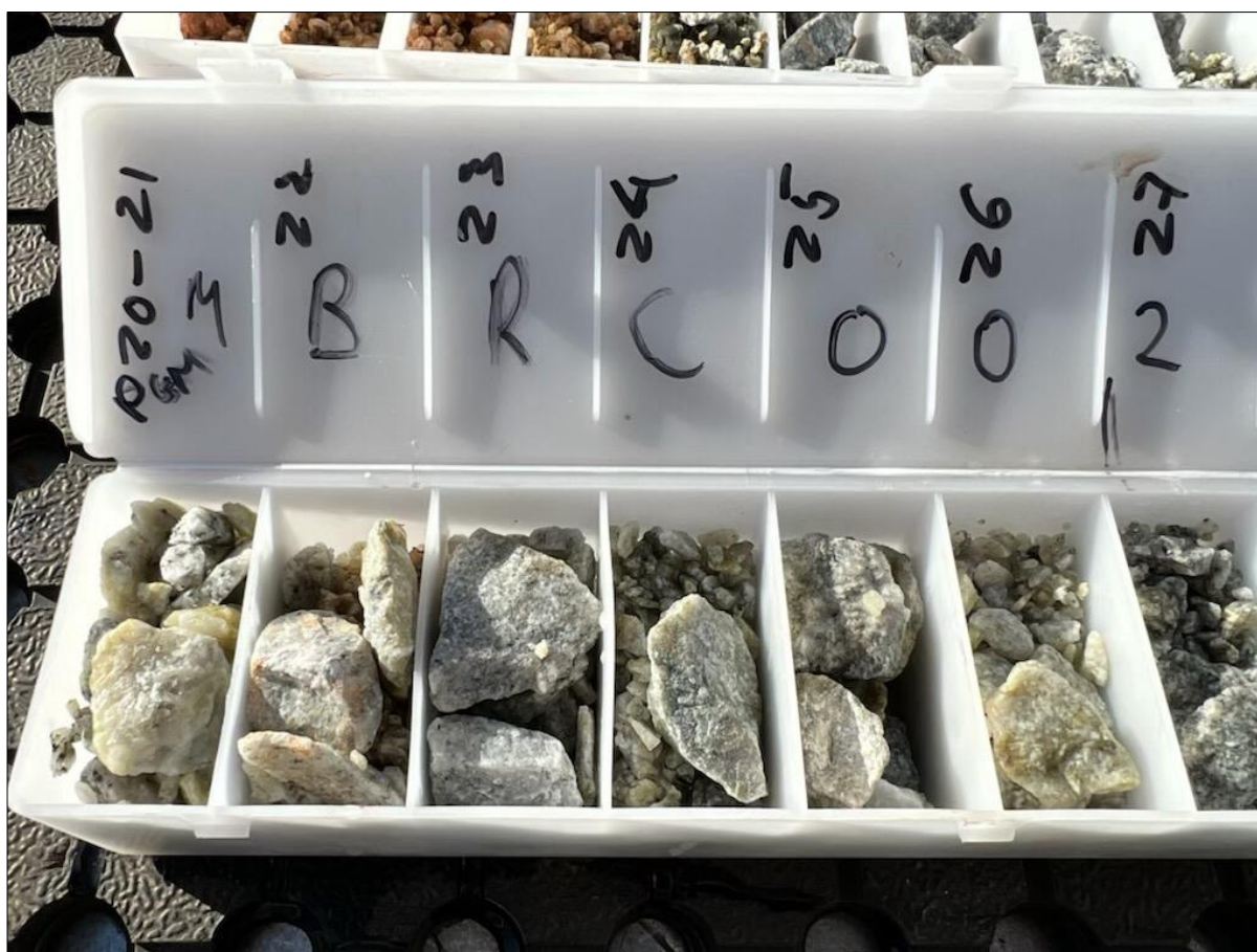
Photo 2 – MBRC002 drillhole intersecting 6 metres of altered Pegmatite from 20m to 26m
