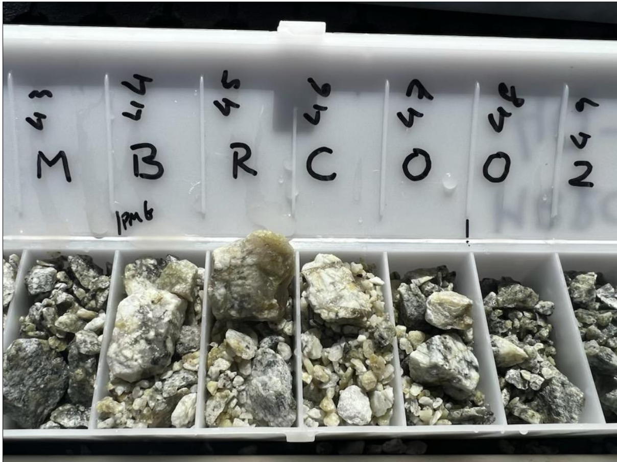
Photo 3 – MBRC002 drillhole intersecting 4 metres of Pegmatite from 44m to 47m
