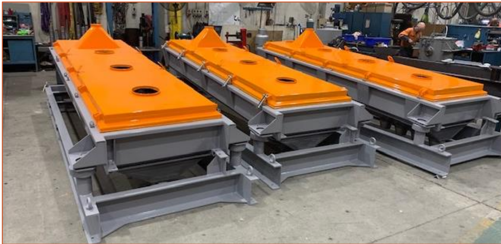
Figure 5: Rotex Screens assembled at the workshop in Melbourne.
