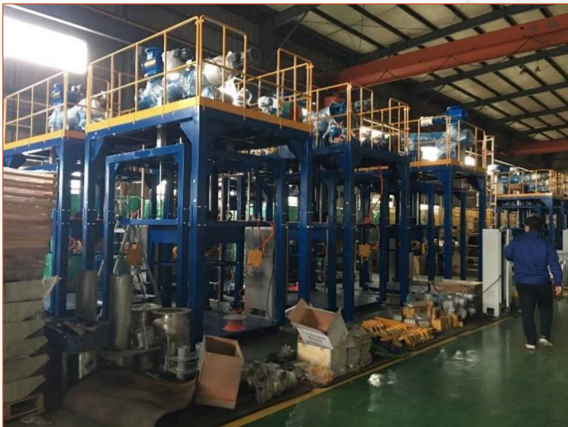
Figure 4: Graphite concentrate bagging equipment undergoing factory testing in China.
