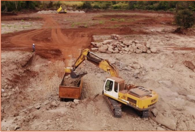
Figure 10: The box-cut being opened with the loading and hauling of the fragmented blasted material in July (left) and the starter pit and temporary high-grade stockpile in mid-August (right).
