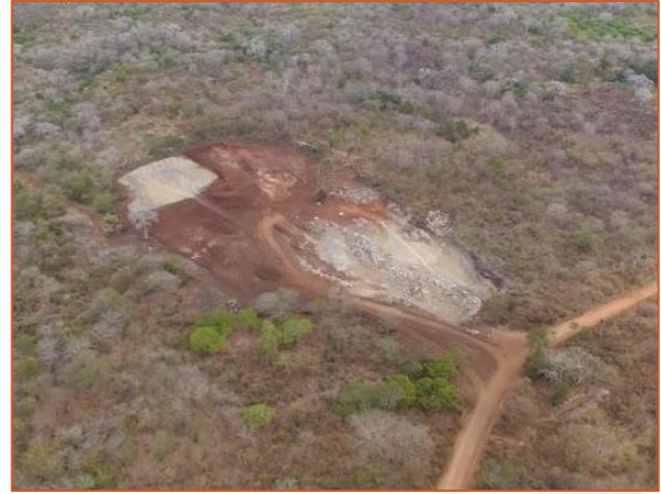
Figure 10: The box-cut being opened with the loading and hauling of the fragmented blasted material in July (left) and the starter pit and temporary high-grade stockpile in mid-August (right).
