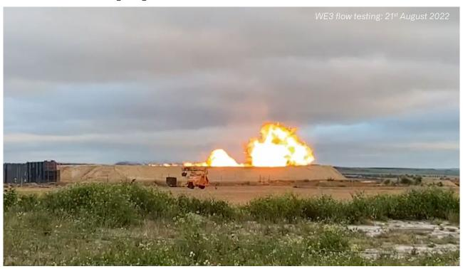
Strike has been testing the producibility from 40m of perforations across the Kingia Sandstone reservoir from 4,733m (measured depth) in the West Erregulla-3 well. Interim results are reflective of the high-quality gas charged reservoir observed in the well's petrophysical analysis.
