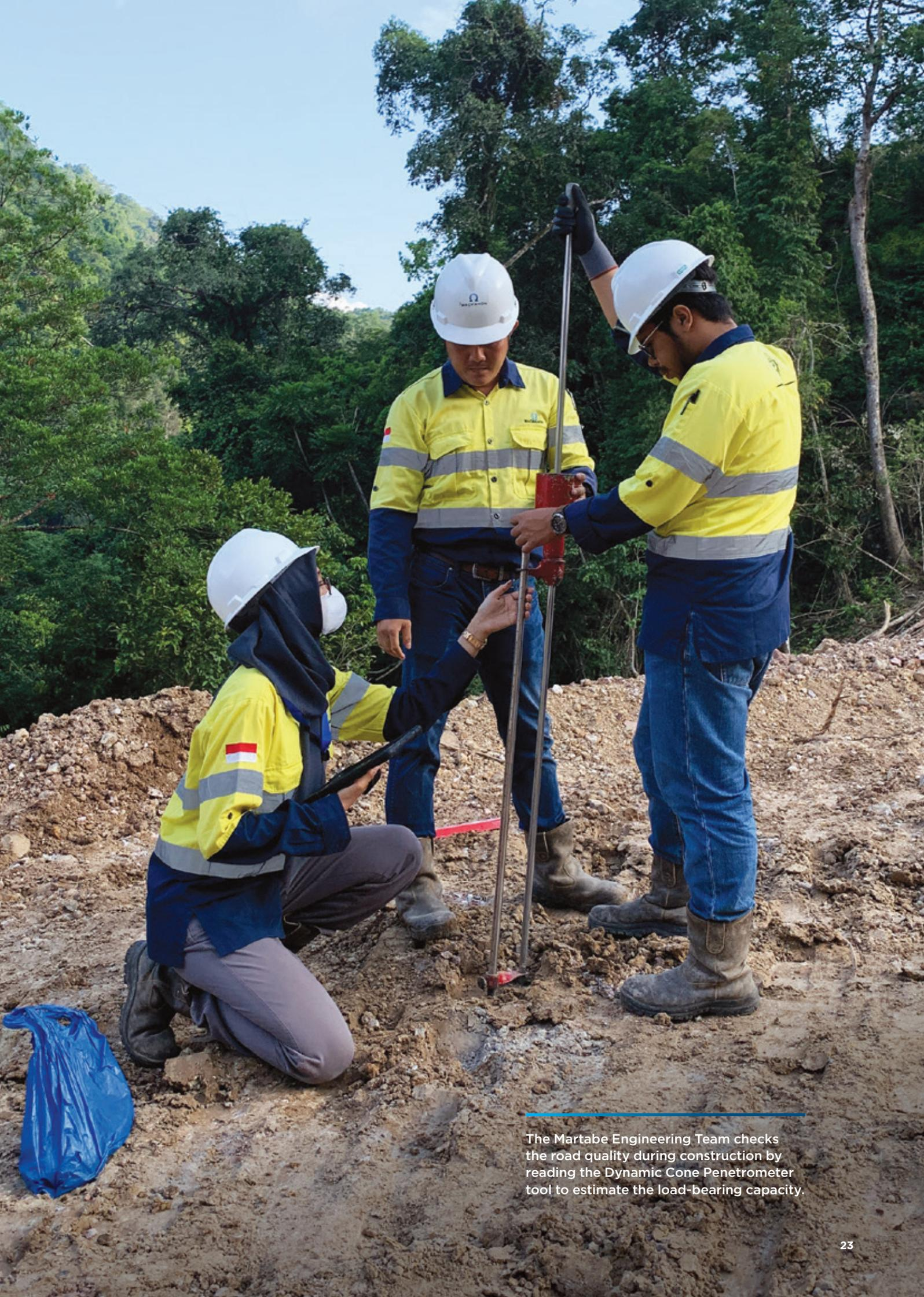
The Martabe Engineering Team checks the road quality during construction by reading the Dynamic Cone Penetrometer tool to estimate the load-bearing capacity.
