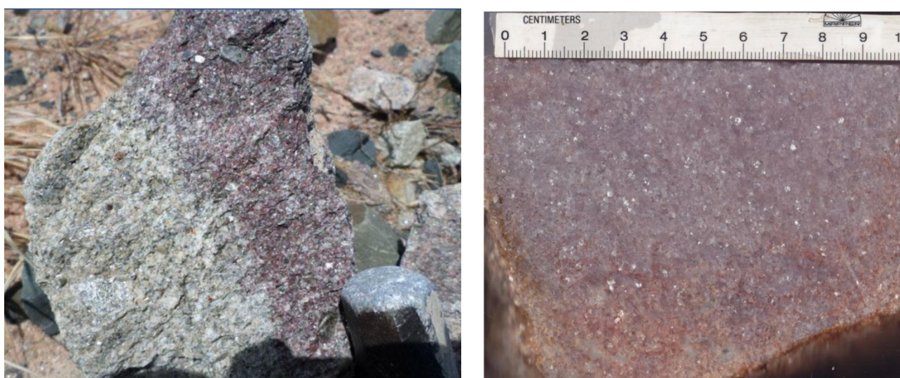
Figure 1. (Left) Sample of red/pink-altered contact with the Blackman Gap granite described as lepidolite (Right) Sample described as lepidolite-rich pegmatite that assayed 3.55% Li 2 O
