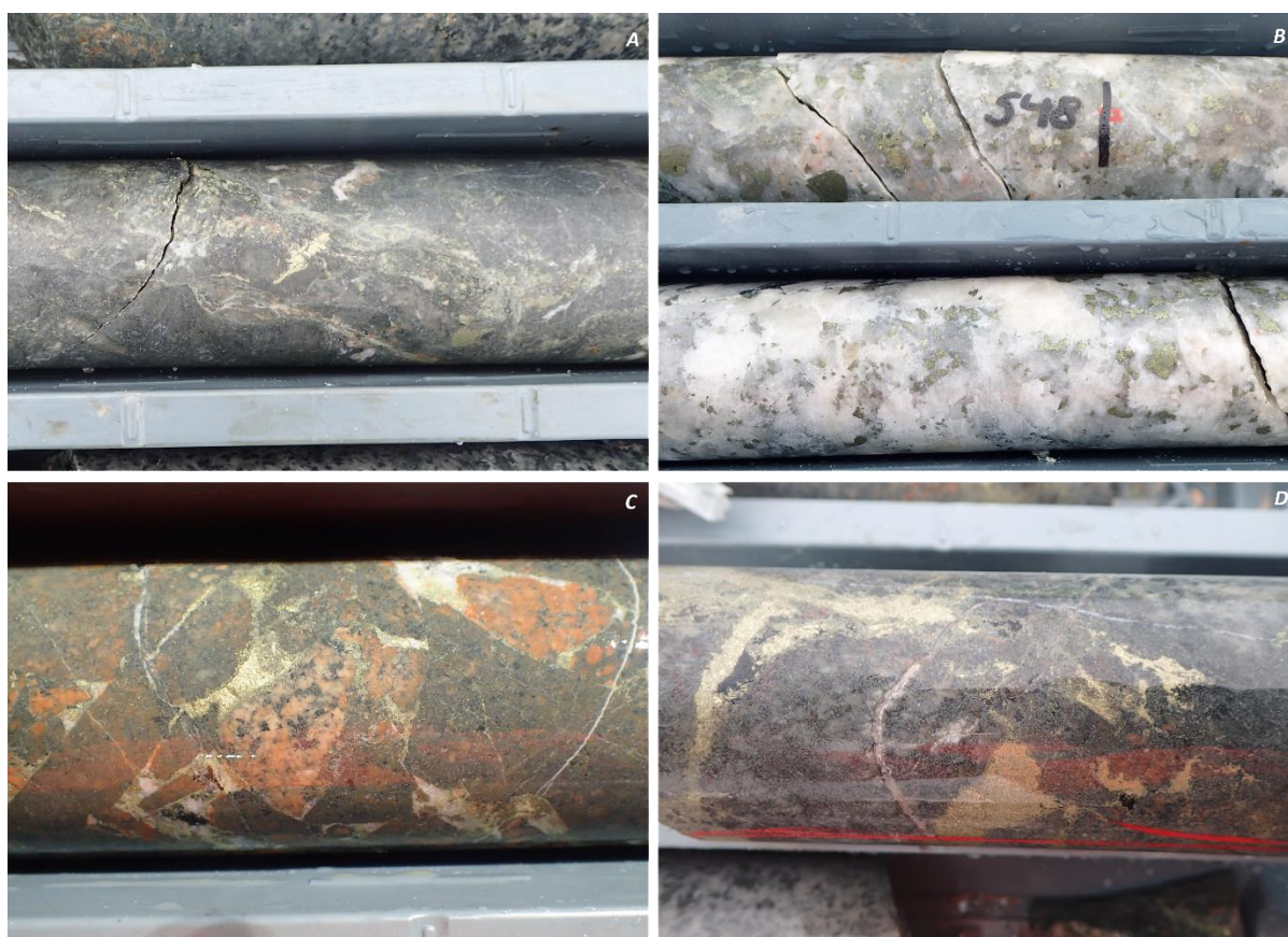
Figure 4. Images of various down hole intervals of HQ drill core (63.5mm diameter) from hole 22MYDD415. A) pervasively chlorite-altered breccia with epidote veining and minor chalcopyrite (yellow, centre) from 402.9m; B) brecciated, low-angle quartz-carbonate vein with large blebs of chalcopyrite (to 20mm) and lesser pyrite from 547.2m; C) K-felspar and chlorite-altered polymict breccia with carbonate-chalcopyrite infill from 574.6m; D) strongly altered diorite breccia with intense chalcopyrite-magnetite infill and minor carbonate veining from 583.3m.
