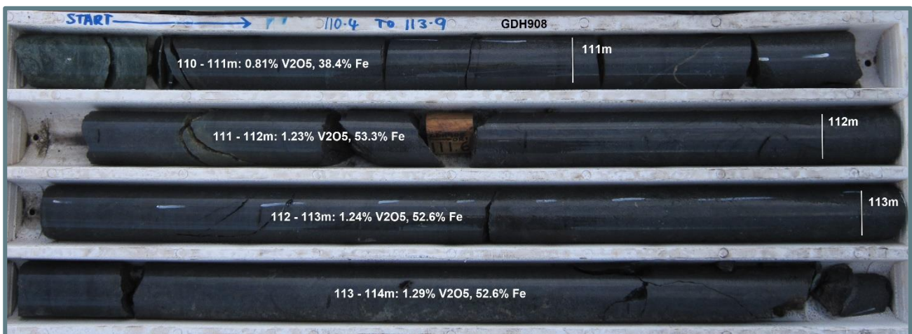
Figure 5 - HG10 domain drill core from GDH908 with V 2 O 5 % and Fe% grades
