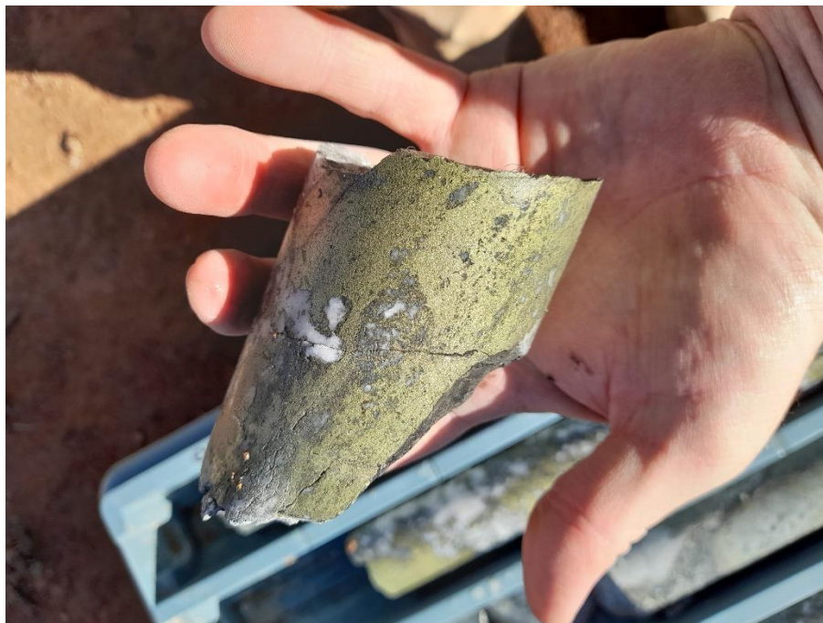
KSNDDH015 - 71.9m: Chalcopyrite vein. Sample interval 71.6m to 72.3m: 5.5% Cu, 0.5g/t Au, 13g/t Ag.
