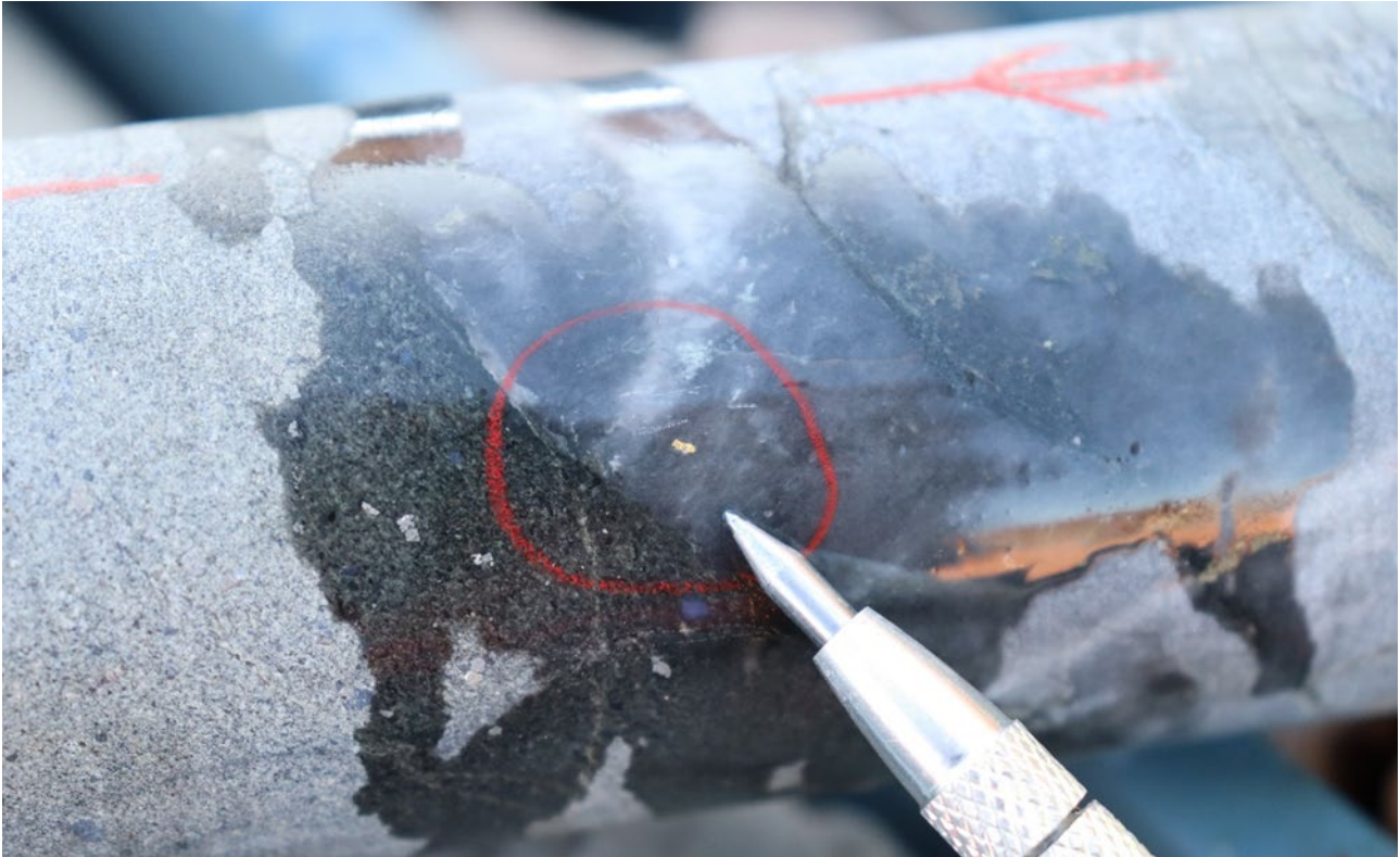
Figure 6: Core photo of 22CYDD004 at Kavanagh intersected quartz veining showing visible gold from 422.71m down hole depth
