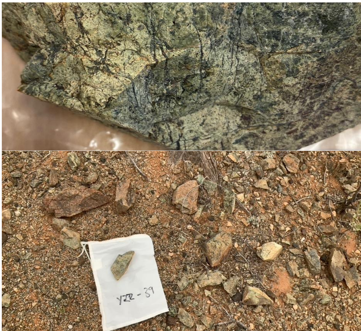
Figure 4: Yinnetharra (WCN 100%) REE/Li project, sample YZZ39 which is highly anomalous in REE's with a grade of 615ppm TREO, and thought to be proximal or near a stronger mineralised source. YZZ39 is proximal to a thorium anomaly that will be sampled in the next field trip expected in the next 2 weeks.
