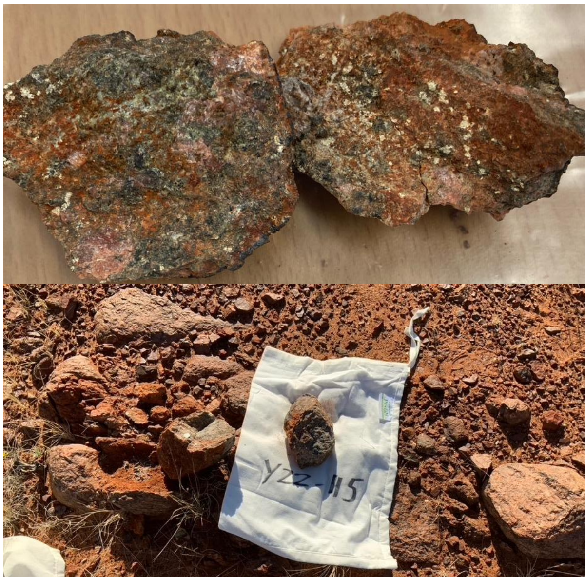
Figure 3: Yinnetharra (WCN 100%) REE/Li project, sample YZZ115 which is highly anomalous in REE's with a grade of 780ppm, and thought to be proximal or near a stronger mineralised source. YZZ115 is proximal to a zone highlighted by reprocessing satellite data which will be more extensively sampled in the next field trip expected in the next 2 weeks.
