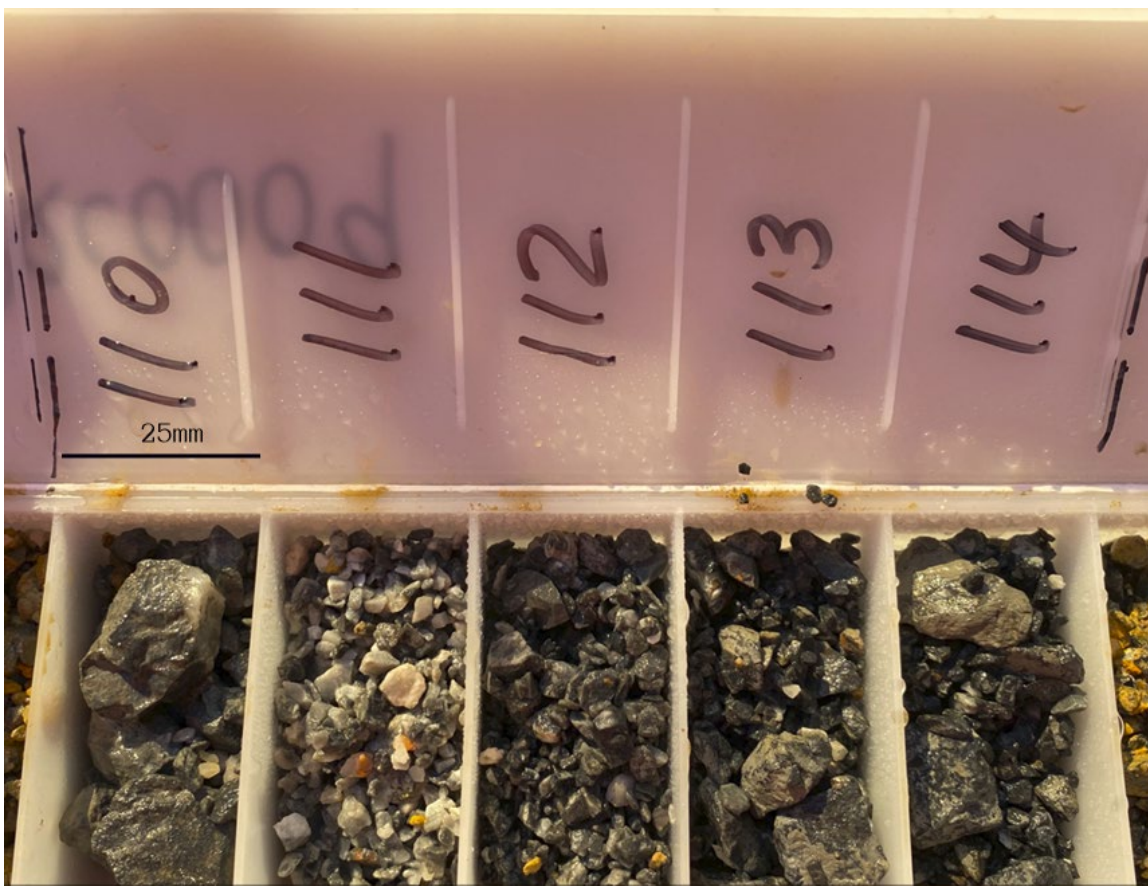
Figure 3: RC chips from PRC0009 exhibiting heavily disseminated sulphides (~30%) with strong silicic alteration
