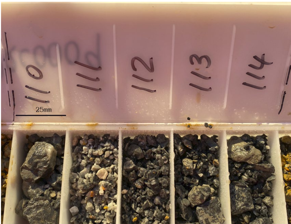
Figure 3: RC chips from PRC0009 exhibiting heavily disseminated sulphides (~30% - predominantly pyrite) with strong silicic alteration
