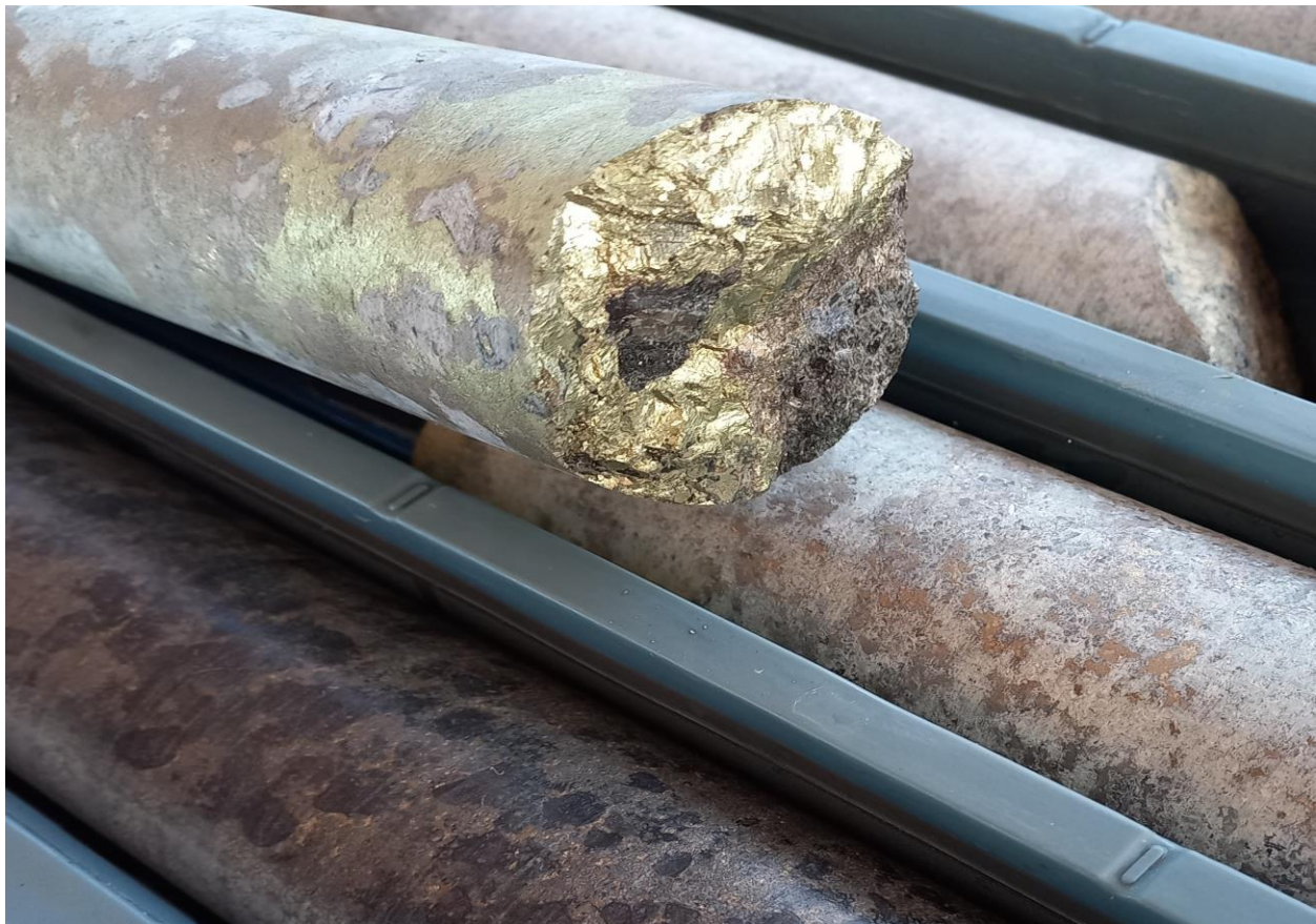
Figure 1: Matrix of copper and nickel sulphides from approximately 561.45m downhole CBDD074
