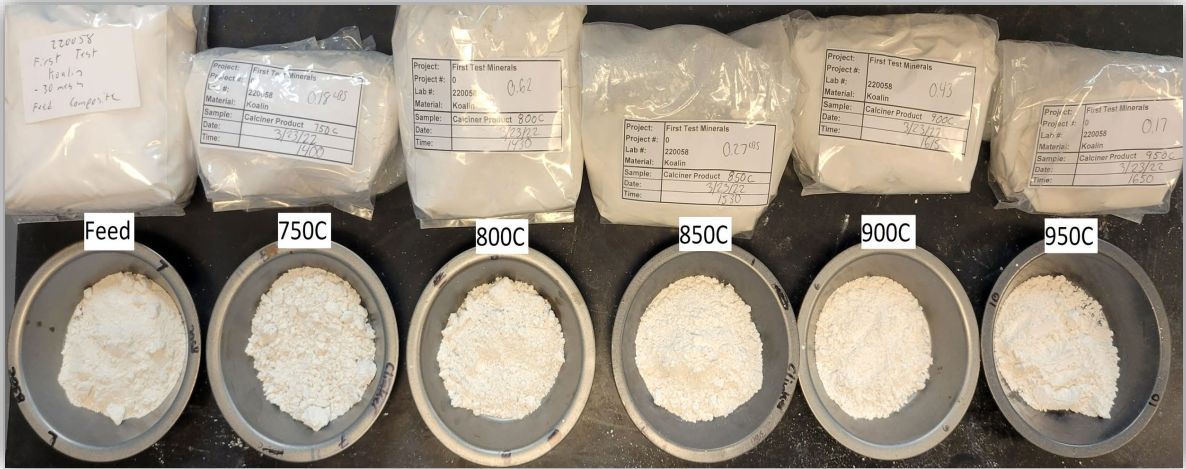
Flash calcined Gabbin hydrous kaolin tested by FLSmidth at various temperatures for suitability for Metakaolin
