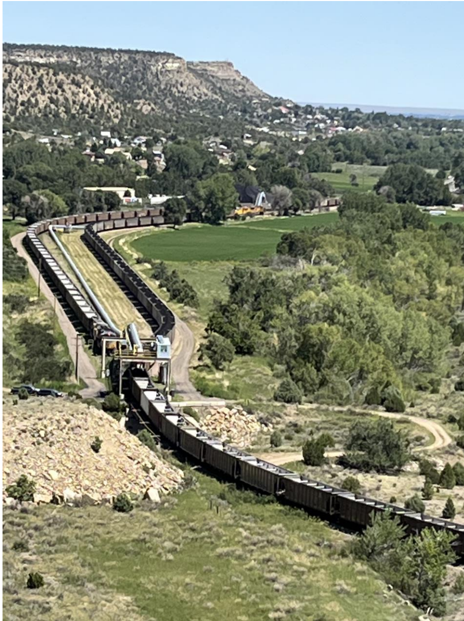
Figure 2: Second Unit Train being loaded at the New Elk Jansen rail Load out facility
