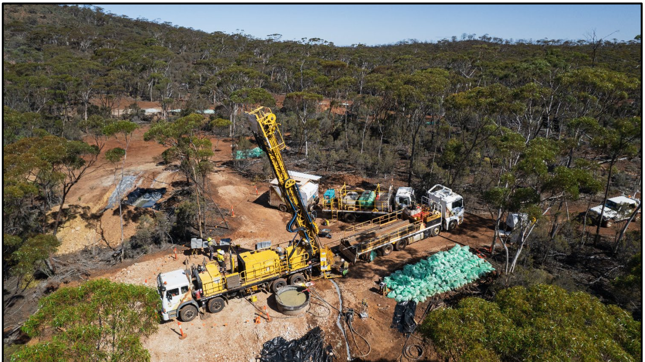
Figure 4 — Diamond core drilling on site at Galileo's 100% owned Callisto discovery near Norseman.
