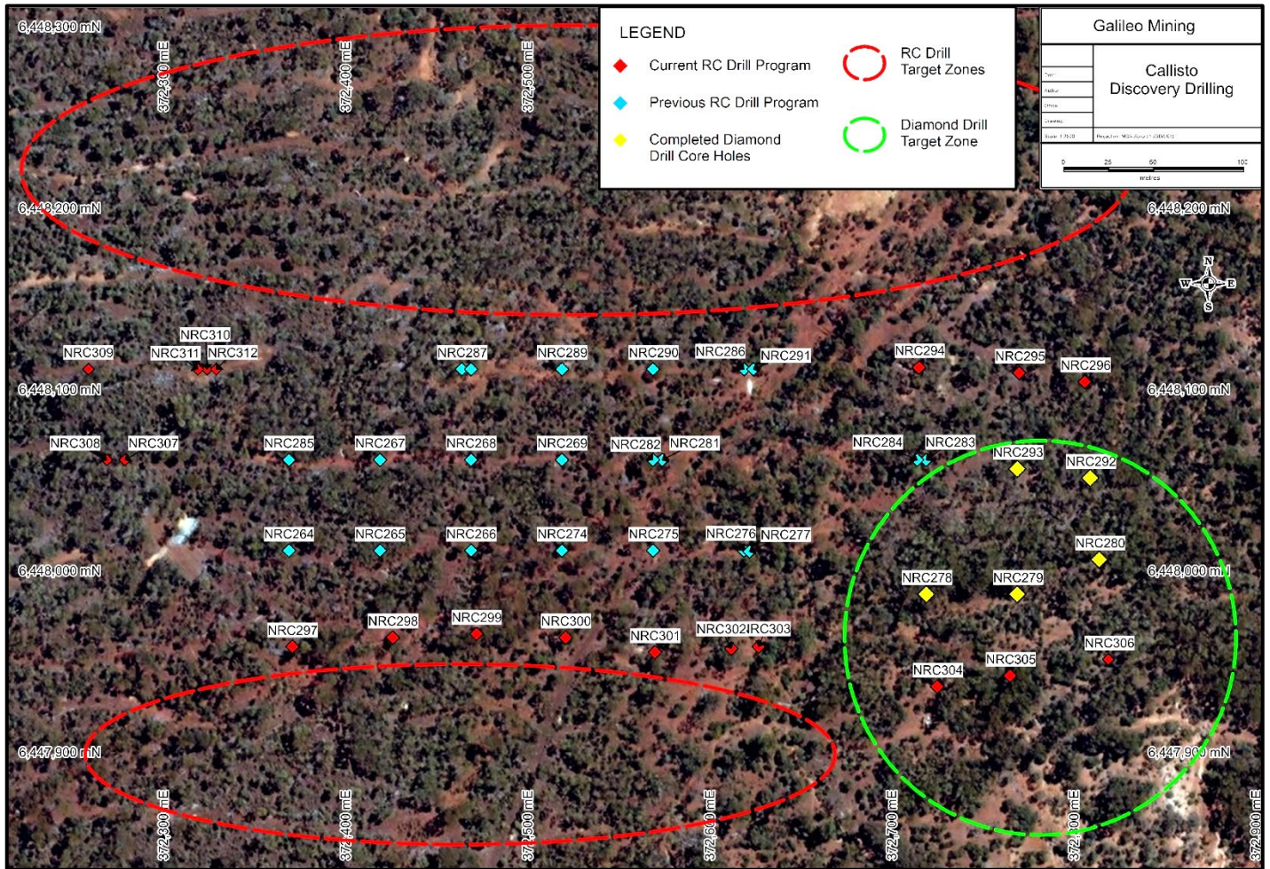
Figure 8 — Plan map of drilling with recently completed diamond drill holes (in yellow) and recent RC drill holes (in red). RC and diamond drill target zones around known sulphide mineralisation for the current drill campaigns are shown (dotted ellipses). Regional RC drilling up to one kilometre away from existing drill holes (off plan to the north) is also scheduled within the current RC program.
