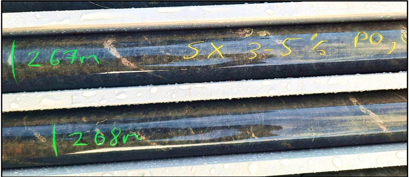
Figure 3 - Disseminated sulphide mineralisation at 267m downhole in NRCD279 (field of view approximately 25cm across). Full core tray photo is in Figure 7. NQ2 core diameter 50.6mm. See Appendices 1,2 & 3 for drill hole details including preliminary visual logging of sulphide mineralisation.
