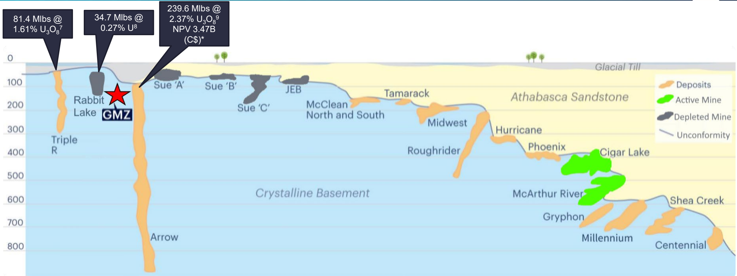
Image: Schematic of Athabasca Basin uranium deposits, basement hosted versus unconformity, and position of Gemini Mineralised Zone
