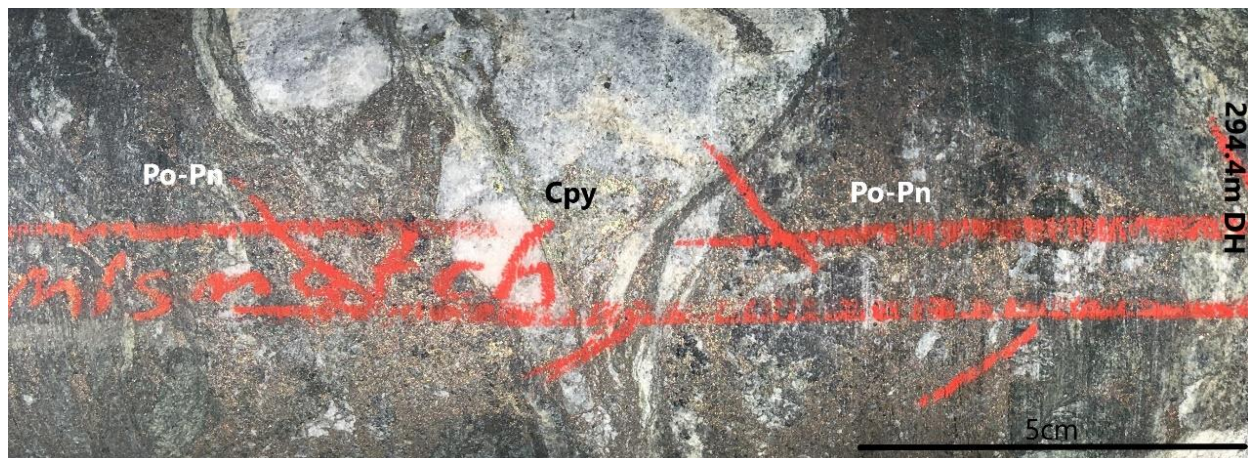
Photo 2: Semi-massive sulphides incl. pyrrhotite (Po), pentlandite (Pn) and chalcopyrite (Cpy) in 22SBD0001
