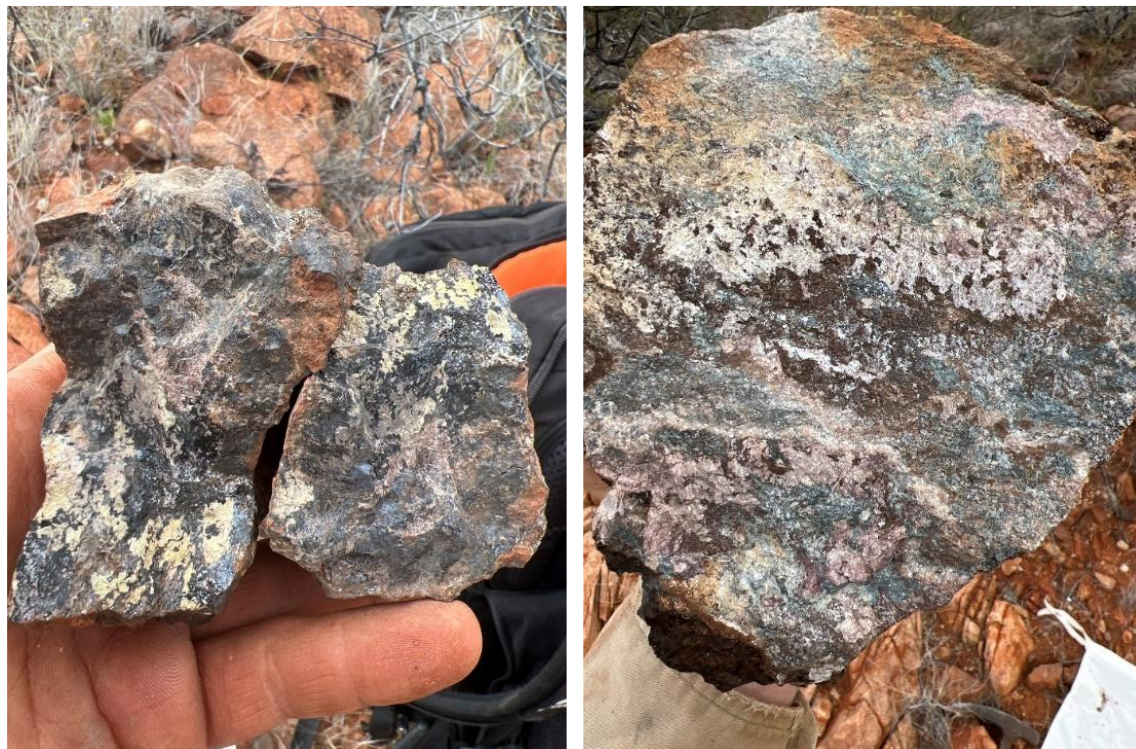
Figure 3: Monazite (pale red) rich carbonatite samples MWGS0769 (left) and MWGS0770 (right) which assayed 21.55% TREO with 3.74% Nd_2O_3 + Pr_6O_{11} and 15.19% TREO with 2.56% Nd_2O_3 + Pr_6O_{11} .
