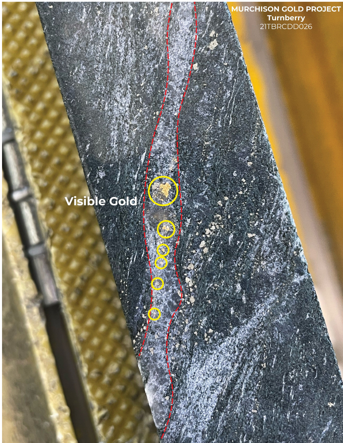
Figure 1: TBRCCDD026 showing nuggetty visible gold within chlorite-pyrite altered dolerite (1m @ 28.23g/t Au from 330m including 0.09m @ 190.85g/t Au).
