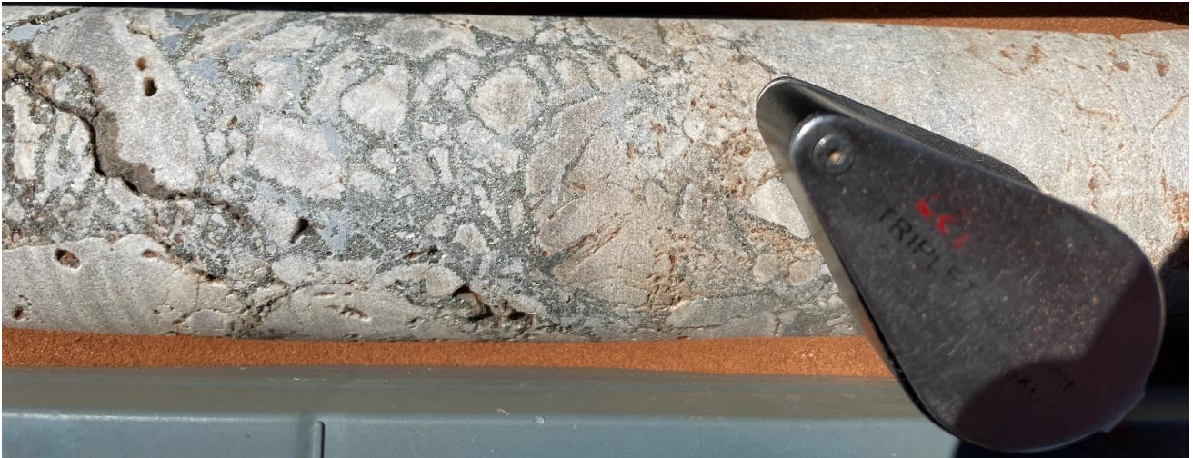
Figure 3: Vuggy and brecciated dolomite interpreted as dolomitised Pillara Limestone intersected at 392.8m in hole BWTDD0001. Note the silvery sulphides infilling the fractures in the dolomite. Core diameter is 47mm.
