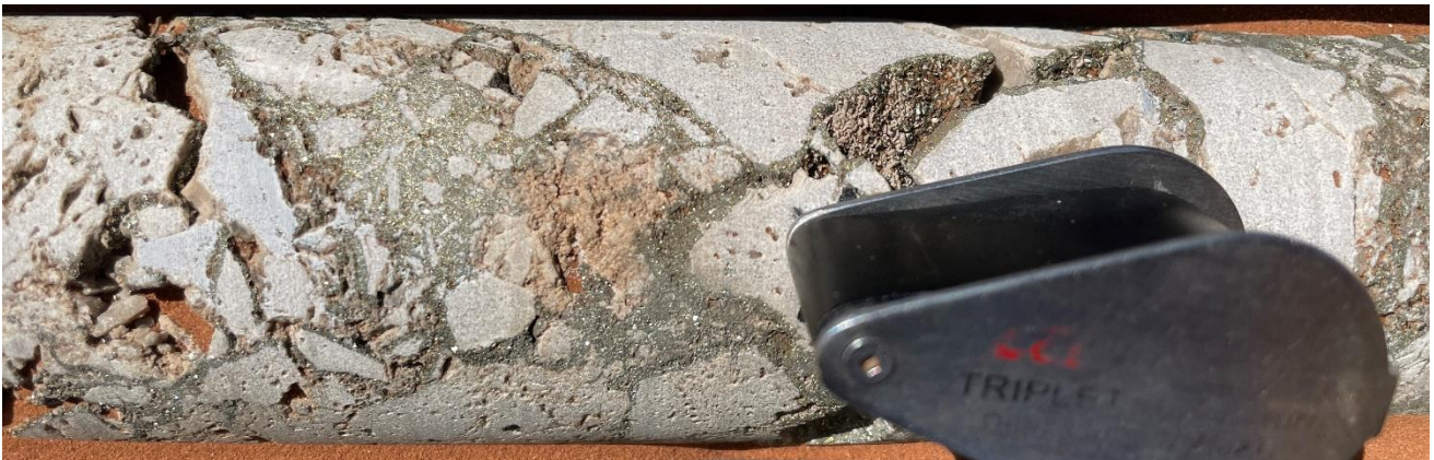
Figure 4: Vuggy and fractured dolomite interpreted as dolomitised Pillara Limestone intersected at 393m in hole BWTDD0001. Note the silvery sulphides infilling fractures in the dolomite. Core diameter is 47mm.
