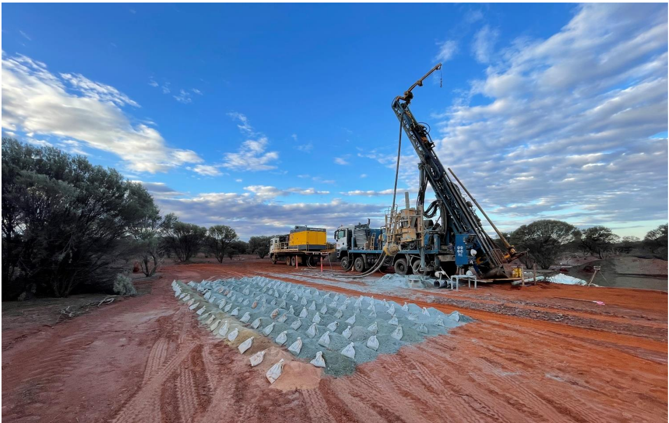
Figure 4: RC drilling and sample layout, Sandstone Gold Project.
