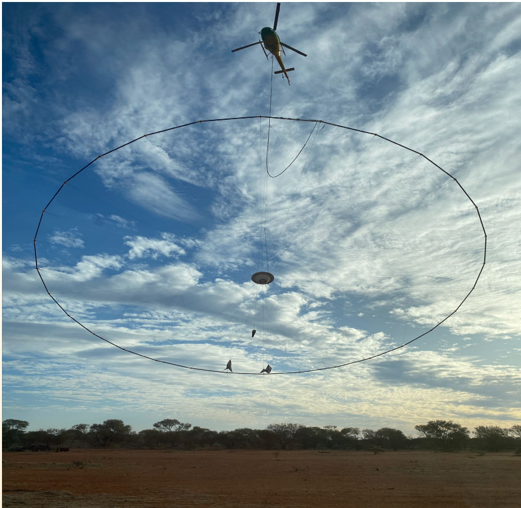
Fig 1. XCalibur Multiscience state-of-the-art HeliTEM 2 system commences Buxton Narryer survey
